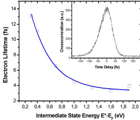
FIG. 3: Spin integrated electron lifetimes (blue squares) and exponential fit (blue line) for intermediate states at  $E^*$  ( $E_g = E^* - 3.1 \text{ eV}$ ). Inset: example bichromatic STR-2PPE cross correlation data used to extract  $n_{\uparrow,\downarrow}$ .
