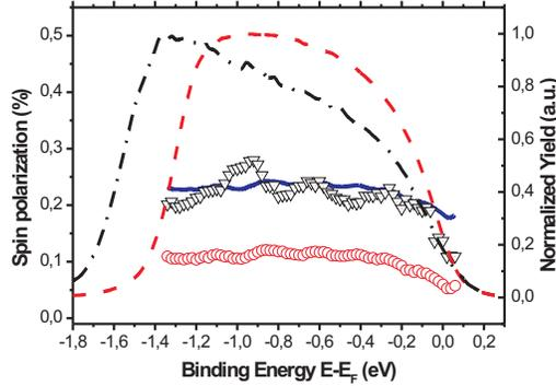
FIG. 2: SP-1PPE (red circles), SP-2PPE (black triangles) and simulated SP-2PPE data (blue full line). The dashed and dotted lines show the corresponding spin integrated 1PPE and 2PPE spectra, respectively.
