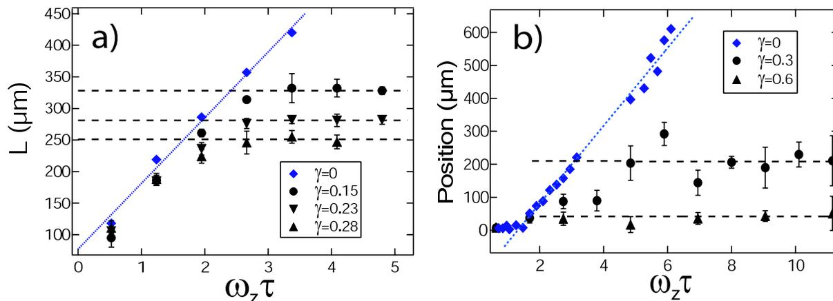
**Figure 7.** *a)* Time evolution of the rms size  $L$  of the expanding Bose-Einstein condensate in the 1D magnetic guide in presence of a 1D random potential with amplitude  $\gamma = \sigma_V/\mu_{\text{TF}}$ . Error bars represents standard deviation over 5 realizations of the speckle pattern (dashed lines are guides to the eye) ; *b)* Time evolution of the centre of mass position for the different values of  $\gamma$ .
