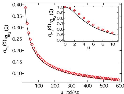
**Figure 2.** Normalized standard deviation  $\sigma_{m_2}(d)/\sigma_{m_2}(0)$  as a function of the length  $d$  of the system. Lozenges  $\diamond$  correspond to the numerical calculation of  $m_2(d)$  with the true auto-correlation function  $C_v(z) = 1 + \frac{\sin[\pi z/\Delta z]}{\pi z/\Delta z}$ . The solid black line represents the analytical solution of Equation (A.10)-(A.11). Inset: shows plot in detail for small values of  $d$ .
