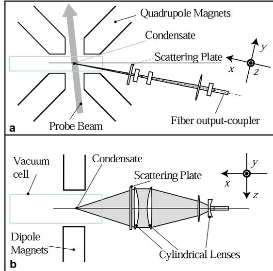
**Figure 3.** Optical setup used to create the speckle potential. The BEC is at the focus of the lens system with its long axis oriented along the  $z$  direction. The two figures are shown in the same scale. The beam incident on the diffuser has different widths in the  $y$  and  $z$  directions, which leads to anisotropic speckle grains (see text). **a)** Side view. **b)** Upper view.
