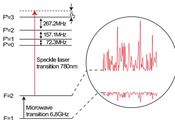
**Figure 4.** The speckle light at 780 nm induces a light shift in both  $F = 1$  and  $F = 2$ . Tuning the speckle laser close to the  $F = 2$  level as shown creates a spatially varying differential light-shift on the 6.8 GHz transition.
