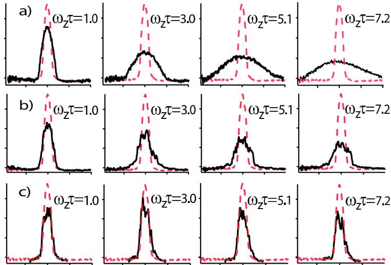
**Figure 8.** Longitudinal density profiles of the expanding BEC for times  $\omega_z\tau = 1.0, 3.0, 5.1$  and  $7.2$  with **a)**  $\gamma=0$ , **b)**  $\gamma=0.15$  and **c)**  $\gamma=0.3$ . The dotted (red) line is the longitudinal profile in the initial trap ( $\tau = 0$ ) in the absence of disorder.
