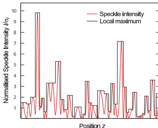
**Figure 6.** Plot of the ‘nearest local maxima’ effective potential (black line) of one realization of the speckle pattern (red line). We use this simulation to obtain the probability distribution of the ‘nearest local maxima’  $P'(I)$ .
