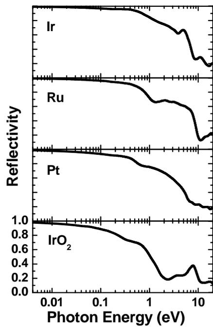
FIG. 1. Reflectance spectra of Ir, Ru, Pt, and IrO<sub>2</sub>.
