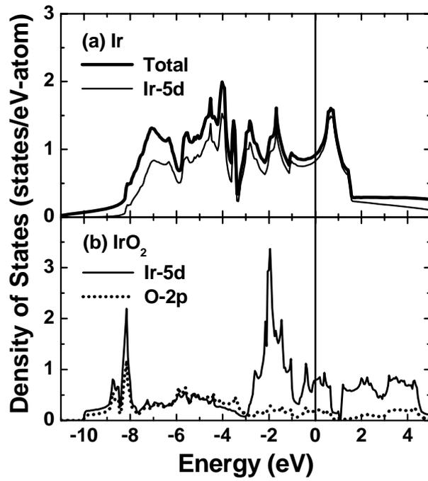
FIG. 6. Density of states (DOS) of (a) Ir and (b) IrO<sub>2</sub>. The thick solid line in (a) represents the total DOS. The thin solid lines in (a) and (b), and dashed lines in (b) represent the projected DOS of Ir-5*d* and O-2*p* states, respectively. Fermi energy was set at zero and is indicated by the vertical solid line.
