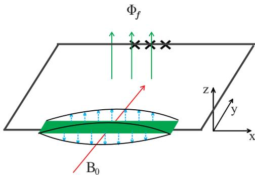
FIG. 1: (Color on line) A 3-Josephson-junction flux qubit loop is located in the  $x$ - $y$  plane and a NAMR is integrated in the loop (indicated by a green line). The  $z$ -direction oscillation of the NAMR couples to the current in the flux qubit loop by a transverse magnetic field  $B_0$  in  $y$ -direction. Another tunable magnetic flux  $\Phi_f$  penetrates this loop tunes the free Hamiltonian of the 3-JJ system.
