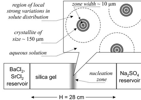
FIG. 1: Experimental setup in which oscillatory zoned crystals of (Ba,Sr)SO<sub>4</sub> were synthesized in Refs. [3, 4, 5]. The reactants counterdiffuse in the column and (Ba,Sr)SO<sub>4</sub> crystals nucleate. The upper window sketches the structure of the nucleation zone and the length scales involved.
