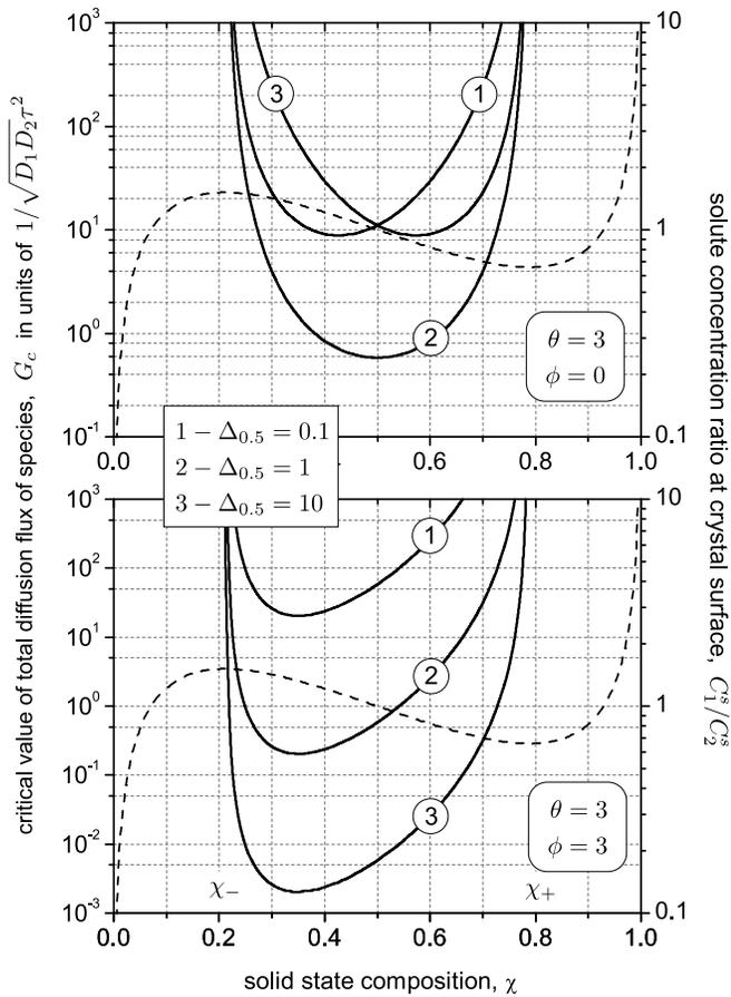
FIG. 4: The critical value of  $G_c$  vs.  $\chi$  for  $\theta = 3$  and some different  $\Delta_{0.5}$  representing the difference in the species solubilities. The upper frame corresponds to a symmetric system with  $\phi = 0$ , the lower one to a strongly asymmetrical one with  $\phi = 3$ . The dashed curves correspond to the function  $N_\chi(\chi)$ .
