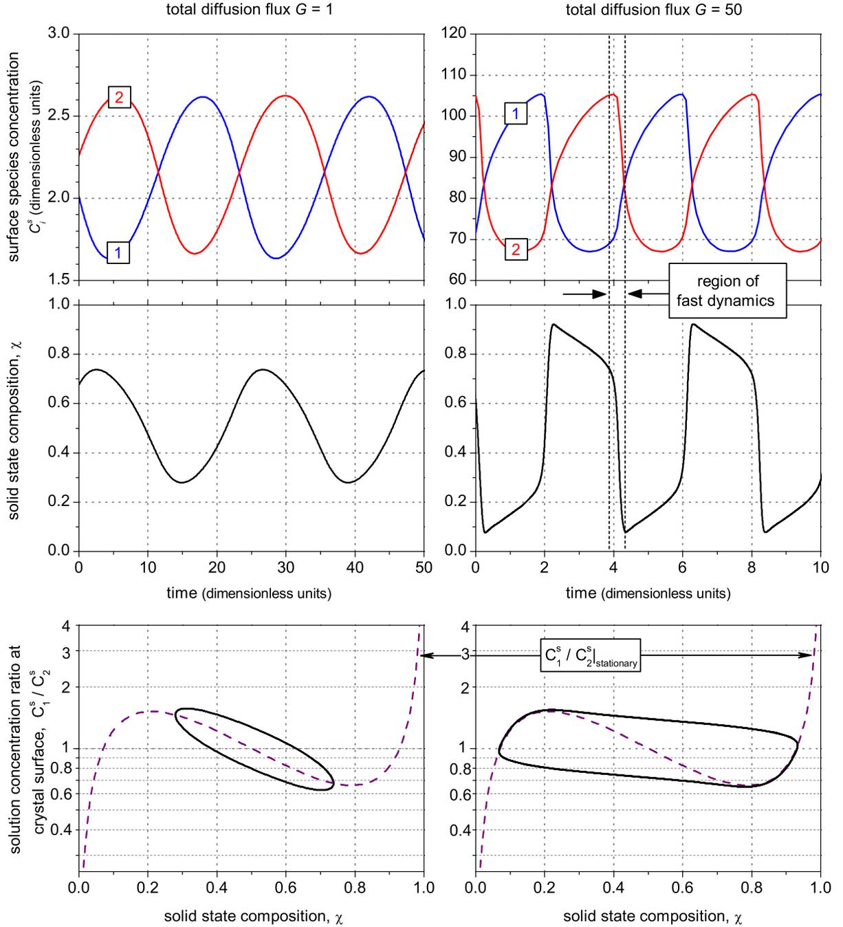
FIG. 5: Dynamics of the symmetrical system  $\theta = 3$ ,  $\phi = 0$ ,  $\Delta_{0.5} = 1$ ,  $\chi_{st} = 0.5$ . The left column has the results obtained for  $G = 1$  which is larger than  $G_c = 0.6$ , see Fig. 4. The right column exhibits the results for  $G = 50$ .
