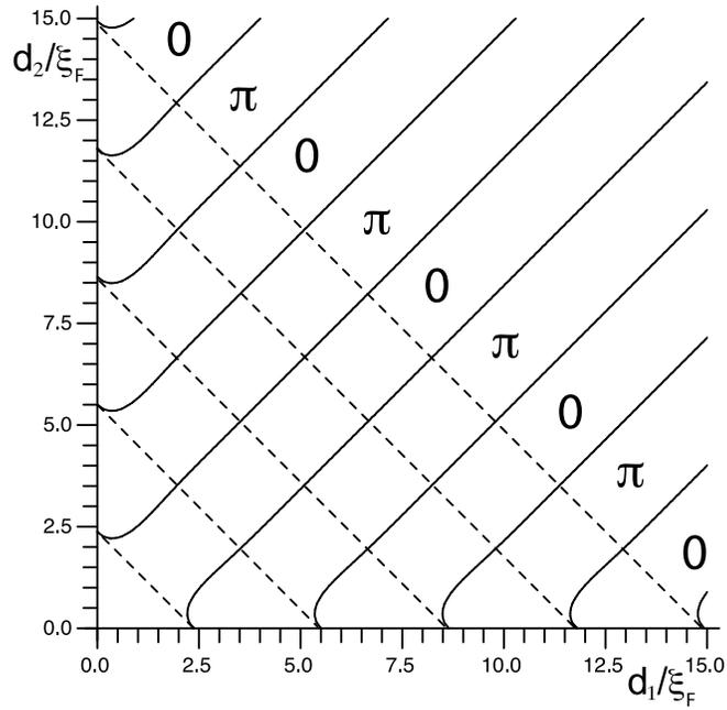
FIG. 2: Quasi-periodic 0 to  $\pi$  transitions for antiparallel (solid lines) and parallel (dashed lines) magnetization. On the graph, the indications 0 and  $\pi$  refer to the antiparallel case. In the parallel case, the transitions occur along lines with  $d_1 + d_2 = \text{const}$ , starting from the 0 state.
