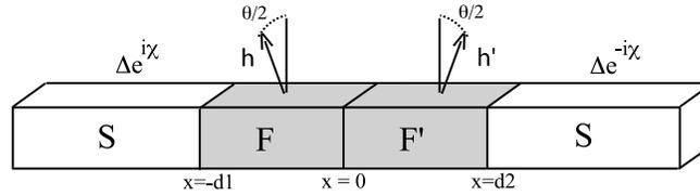
FIG. 1: S-FF<sup>0</sup>-S junction with non-collinear magnetization.
