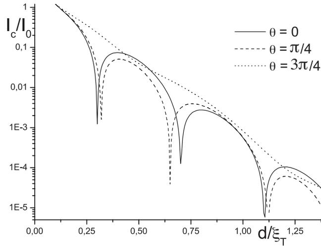
FIG. 3: Critical current dependence on the size of the junction for  $\theta = 0$ ;  $\theta = \pi/4$  and  $\theta = 3\pi/4$ . We take  $h=T = 100$  which corresponds to a realistic value for a diluted ferromagnet, as reported in Ref. 11 and  $\xi_T = \sqrt{D} = 2 \xi$ .
