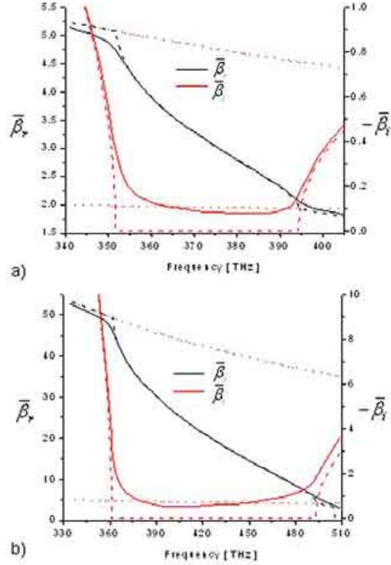
Figure 11 – (Color online). Similar to Fig. 9 and 10, but in a *Si* background ( $\epsilon_{Si} = 14.6 \epsilon_0$ ). In (a):  $a = 10 \text{ nm}$ ,  $d_z = d_y = 22 \text{ nm}$ ,  $d_x = 3d_y$ ; in (b)  $a = 1 \text{ nm}$ ,  $d_z = d_y = 2.2 \text{ nm}$ .
