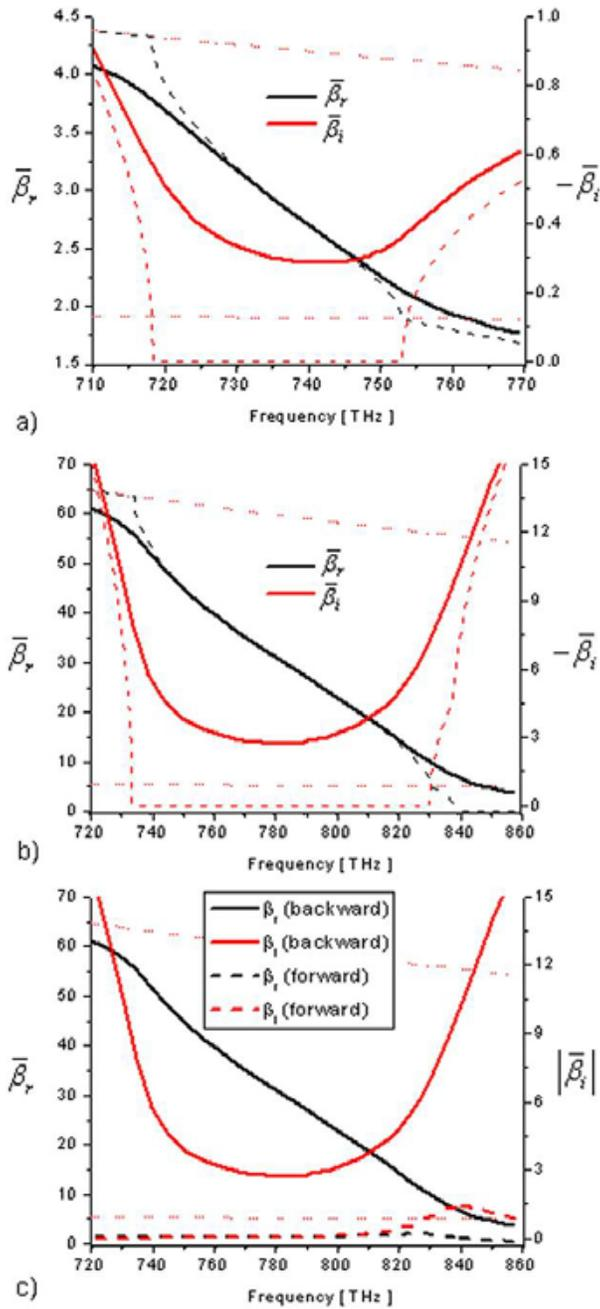
Figure 9 – (Color online). Dispersion plots of the negative-index operation versus frequency for a metamaterial made of silver particles, using silver material parameters (including losses) from experimental data for its bulk properties from [48], in a glass background ( $\epsilon_{SiO_2} = 2.14 \epsilon_0$ ). The
