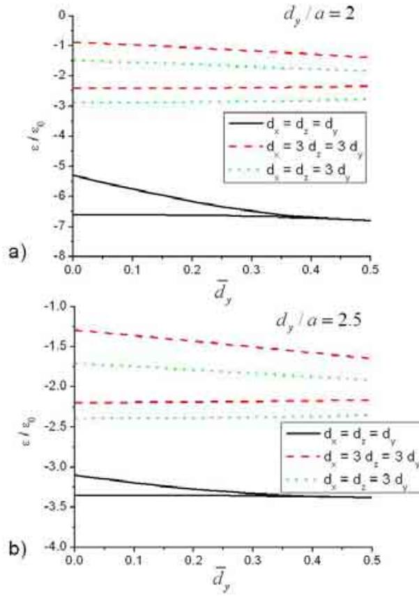
Figure 4 – (Color online). Regions of negative-index operation in terms of the permittivity of the spherical particle and their relative spacing factors in the three directions.
