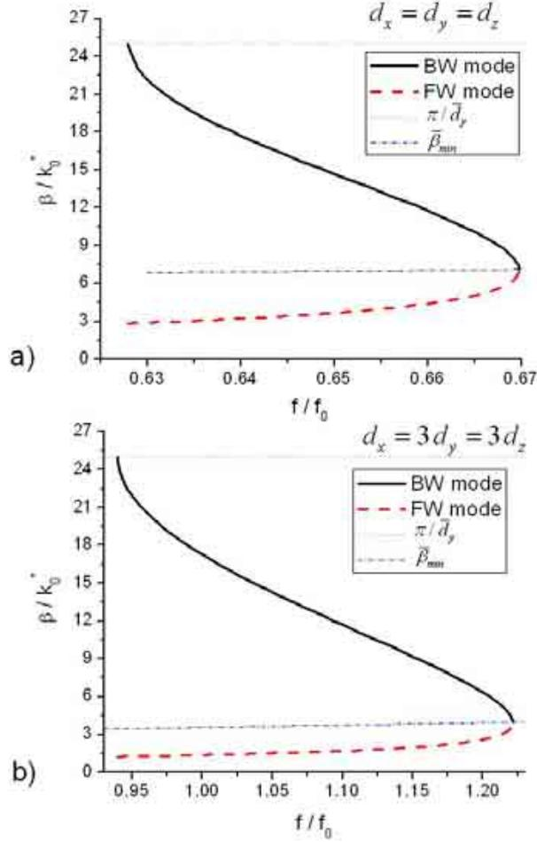
Figure 5 – (Color online). Normalized wave number  $\beta$  (with respect to  $k_0^* = 2\pi f_0 \sqrt{\epsilon_0 \mu_0}$ ), vs. normalized frequency  $f/f_0$ , for TE propagation in a metamaterial made of plasmonic spheres with radius  $a = \lambda_0/100$  (at frequency  $f_0$ ), and center-to-center distance  $d_y = 2.1a$ . The sphere permittivity is assumed to follow a Drude dispersion model with  $\epsilon(\omega) = \epsilon_0(1 - 3f_0^2/f^2)$ .
