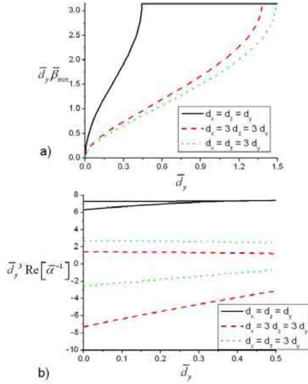
Figure 3 – (Color online). (a) Variation of the minimum value of  $\bar{\beta}_y$  for achieving a backward-wave propagation, in terms of  $\bar{d}_y$ , for different values of the other spacing factors; (b) corresponding region of polarizabilities for which TE backward-wave propagation is supported.
