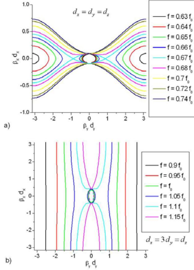
Figure 15 – (Color online). Equipfrequency dispersion curves of the normalized wave vector  $\bar{\mathbf{\beta}}$  in the longitudinal plane (longitudinal with respect to the polarization of the field) for a metamaterial made of spheres with radius  $a = \lambda_0 / 100$  and spacing  $d_y = 2.1a$  at the frequency  $f_0$ , with homogeneous permittivity of the particles following a Drude dispersion  $\varepsilon(\omega) = \varepsilon_0(1 - 3f_0^2 / f^2)$ .
