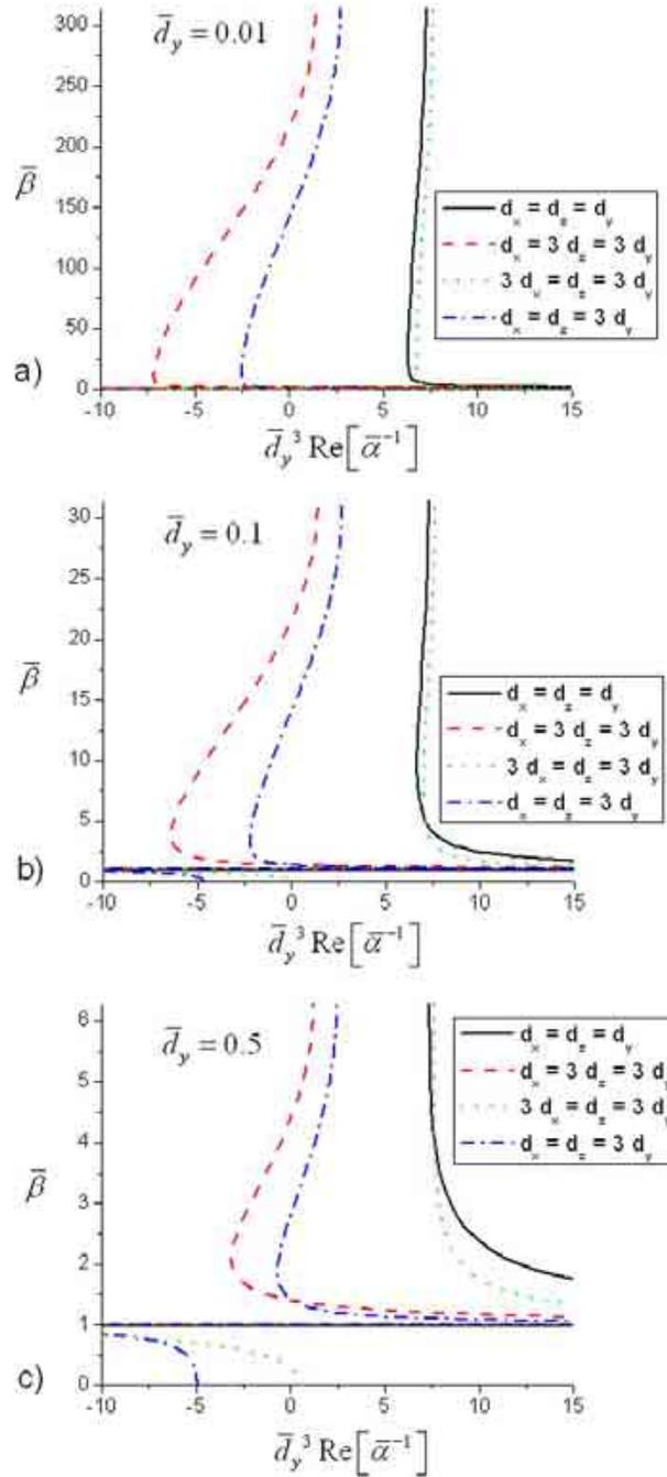
Figure 2 – (Color online). Normalized wave numbers versus normalized inverse polarizability for TE propagation (in this case  $\beta_x = \beta_z = 0$  and  $\mathbf{p}_{lmn} = p e^{im\beta_y d_y} \hat{\mathbf{x}}$ ) for different values of the distance between neighboring particles.
