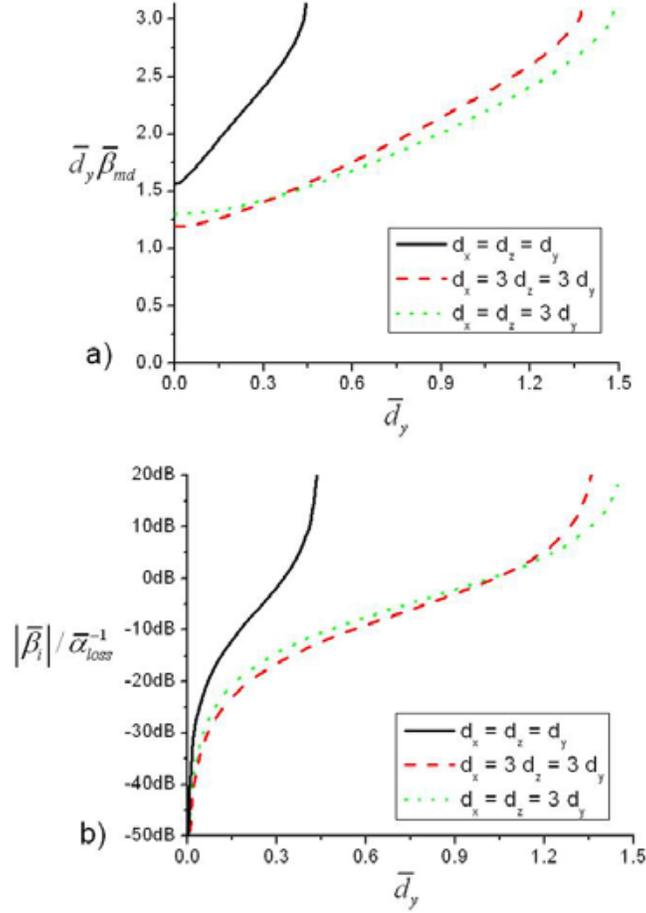
Figure 7 – (Color online). (a) Behavior of  $\bar{\beta}_{md}$  (satisfying Eq. (10), normalized to  $\bar{d}_y^{-1}$ ) versus the normalized longitudinal distance  $\bar{d}_y$  between neighboring particles; (b) Normalized attenuation factor,  $|\bar{\beta}_i| / \bar{\alpha}_{loss}^{-1}$ , for  $\bar{\beta}_y = \bar{\beta}_{md}$ , i.e., variation of the minimum attenuation factor for a given material loss factor  $\bar{\alpha}_{loss}^{-1}$ .
