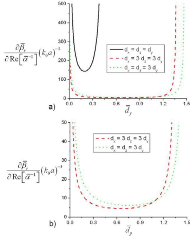
Figure 8 – (Color online). Attenuation factors (as in Fig. 7b, but normalized to the factor  $(k_0 a)^3$  that takes into account of the increase in the loss coefficient when the particle size is reduced, as
