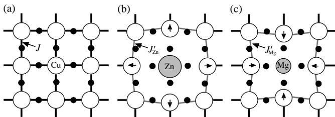
Fig. 2. Schematic representations of (a) a  $\text{CuO}_2$  plane, where the small closed circles represent positions of oxygens, (b) a  $\text{CuO}_2$  plane with Zn-substitution, and (c) a  $\text{CuO}_2$  plane with Mg-substitution.
