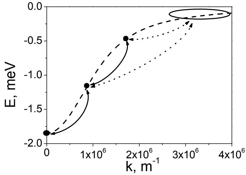
Figure 1. Schematic diagram of parametric amplifier with reservoir. The dashed line is the lower polariton dispersion. The black circles on the line are the signal pump and idler state respectively. The solid line arrows are sketching the parametric polariton scattering process. The dotted arrows show the phonon induced transfer between the idler state, the pump state and the excitonic reservoir.
