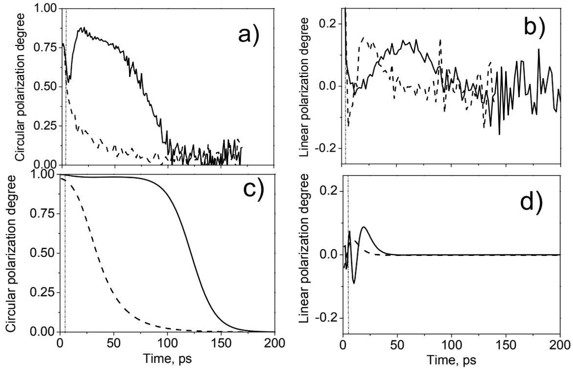
Figure 4. Circular and linear polarization degree of the signal emission for elliptically polarized pumping: experiment (a, b) and theory (c, d). Dashed line corresponds to  $0.5 \text{ W/cm}^2$  (below threshold) and solid line corresponds to  $3 \text{ W/cm}^2$  (above threshold). Note that the initial polarization peak in (a,b) is due to diffusion of the excitation pulse on the sample surface.
