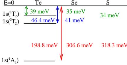
FIG. 1: (Color online) First ionization energies of the 1s levels of double donors (Te, Se, S) in Si. The ground state is the singlet  $1s(^1A_1) = [1s(A_1), 1s(A_1)]$  and the first excited states are  $1s(^i T_2) = [1s(A_1), 1s(T_2)]$ . ( $i = 1$ ) corresponds to a singlet while ( $i = 3$ ) to a triplet. Data taken from Refs. 10, 11.
