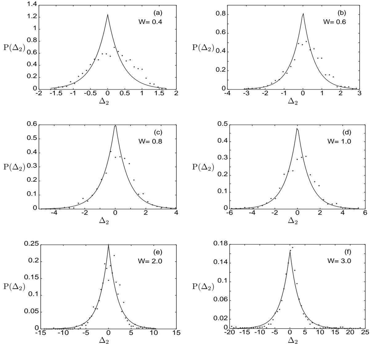
**Figure 4.** Comparison of numerical results and the two-sided exponential function for the CELS function  $P(\Delta_2)$ .  $W$  is a measure of the disorder. At small  $W$ ,  $P(\Delta_2)$  is approximately Gaussian, but for  $W > 2$  the two-sided exponential fit is better, suggesting the start of a crossover.
