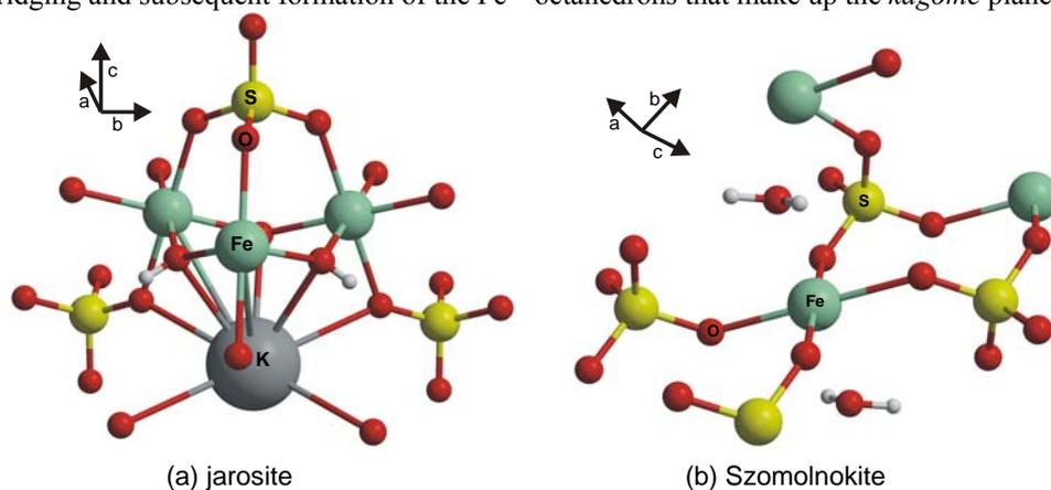
Figure 3(a). Structural representation of the jarosite structure. The sulphate groups cap above and below the Fe octahedra sitting along the 3-fold axis. Each of these subunits is separated by the A-site, K<sup>+</sup> in the diagram. (b) Szomolnokite has a more open structure; the distortion from rhombohedral is only slight:  $\beta \sim 120^\circ$  and the a and b lattice parameters are similar to the a parameter in jarosite.
