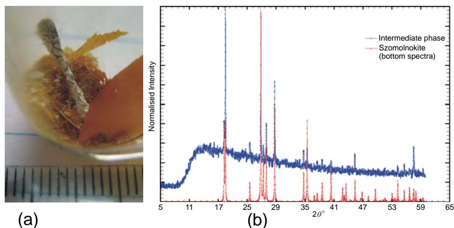
Figure 2(a). Photograph of Szomolnokite (white) growing on the surface of the Fe wire. The image captured through a Pyrex tube also shows the dark ochreous colour of potassium jarosite surrounding the Fe wire. (b) The diffraction spectrum of the intermediate phase (top spectra) matched with that of synthetic Szomolnokite -  $\text{Fe}^{2+}(\text{SO}_4) \cdot \text{H}_2\text{O}$  (bottom spectra) calculated with FullProf from the crystallographic data given in Table 1.
