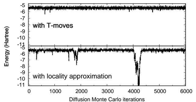
FIG. 1: Energies for the Carbon pseudoatom with  $\tau = 0.08H^{-1}$  at the given DMC generation.  $\Psi_T$  is an antisymmetrized geminal power (AGP) wave function with a 3-body Jastrow factor[12, 15]. We report results for the locality approximation ( $H^{\alpha,\gamma}$  with  $\alpha = 1$  and  $\gamma = 0$ ) and the algorithm with  $T$ -moves ( $\alpha = 0, \gamma = 0$ ).
