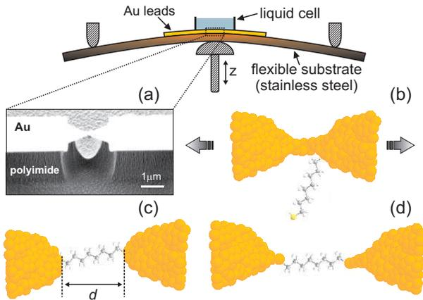
Figure 1: (a) Schematics of the MCBJ principle with liquid cell and a SEM image of one underetched Au junction. (b)-(d) Principle of the formation of a metal-molecule-metal bridge during the breaking process. Starting from the fused Au leads (b), a molecule can lock between the leads (c). Under further stretching, the Au leads are deformed, while the Au-octanedithiol-Au junction stays intact (d).
