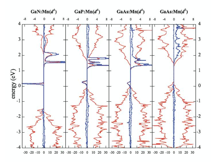
FIG. 3: The spin-resolved total DOS (solid red line and bottom scale) and Mn-DOS (dotted blue line and top scale) from left to right, for  $Mn-d^4$  impurity in GaN, GaP, and GaAs, as well as  $Mn-d^5$  impurity in GaAs. Results are shown for 64 atom supercell (3.125% Mn).
