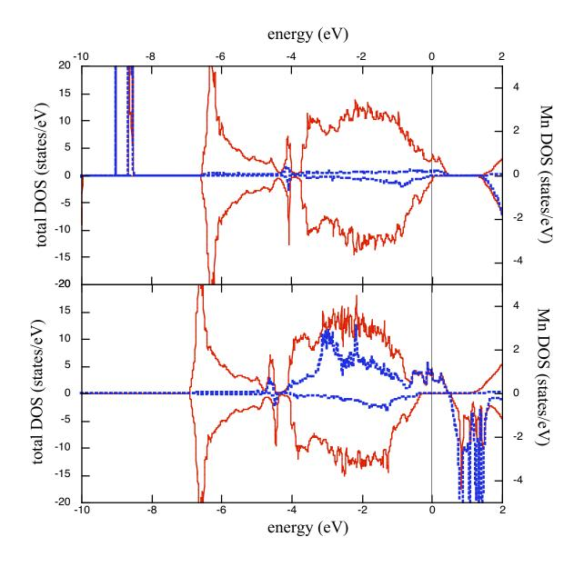
FIG. 1: The spin-resolved total DOS (solid red line) and Mn partial DOS (dotted blue line) of  $(Ga_{1-x}Mn_x)As$  with x = 6.25% for the SIC-LSD ground state,  $d^5$ , scenario (upper panel) as well as the LSDA (lower panel).
