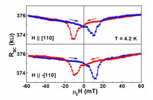
FIG. 3 Electrical resistance  $R_{BC}$  measured between terminals of the arms B and C of the device as a function of a magnetic field oriented along the arm A swept in two opposite directions (differentiated by triangles or circles). The magnetic field direction in the lower plot was reversed with respect to the case of the upper plot. No "remnant resistance" appears.
