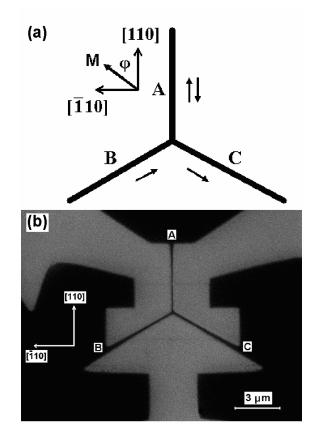
FIG. 1 Three-arm nanostructure: (a) Schematic view where arrows represent magnetization vectors, (b) scanning electron microscope image where darker contrast corresponds to the non-etched conducting areas of the structure.
