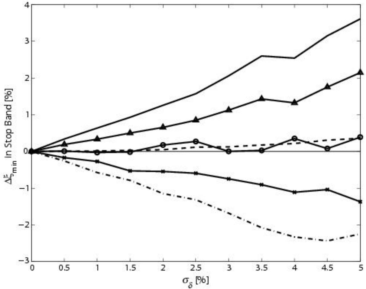
Figure 25 Sensitivity distribution quantities pertaining to the change of frequency spectrum characteristics (i.e.,  $\Delta\xi_{\min}^{\xi}$  at  $\Omega^* = 20$ ) as a result of statistical variations in layer thicknesses of unit cell ‘0101010101’ (see Fig. 2). (—) Maximum, (---) Average, (- · -) Minimum, (—▲—) 95th percentile, (—○—) 50th percentile, (—×—) 5th percentile.
