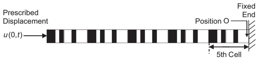
Figure 12 Banded structure designed for achieving shock isolation over frequency range  $0 \leq \Omega^* \leq 50$ . The structure is formed from the synthesized unit cell encoded '0010110111', shown in Fig. 2. Its length is  $L = 5$ . The excitation  $u(0,t)$  is given by Eqs. (28)-(29). Position O marks a measurement point.
