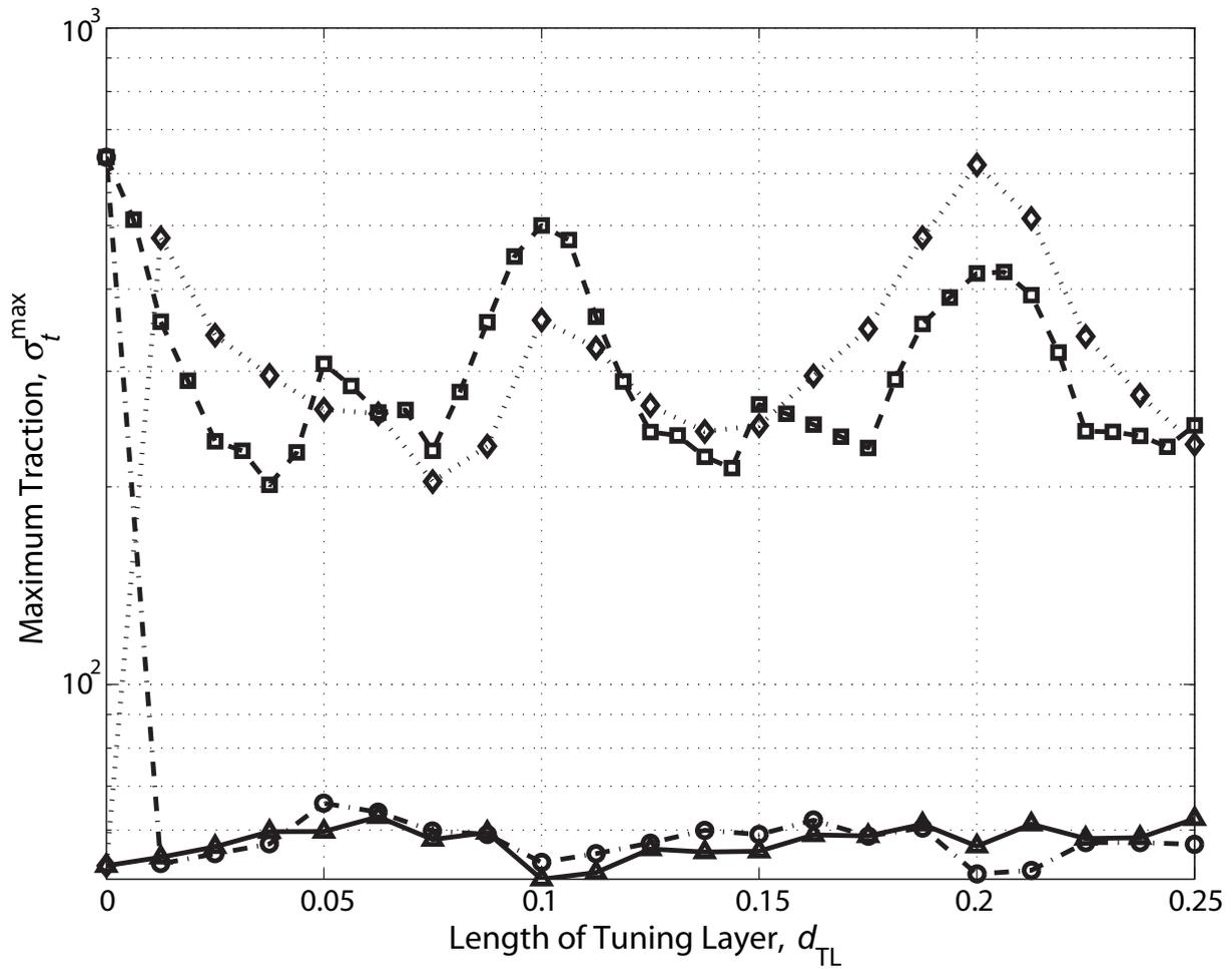
Figure 6 Maximum transmitted traction at right (receiving) end versus length of tuning layer, for different layer ordering and different tuning layer material type. A binary encoding scheme is used to represent the layered unit cell. Stiff and compliant tuning layers are denoted “/Stiff” and “/Compliant”, respectively. (—○—) ‘0101010101’/Stiff, (—□—) ‘0101010101’/Compliant, (—△—) ‘1010101010’/Stiff, (···◇···) ‘1010101010’/Compliant.
