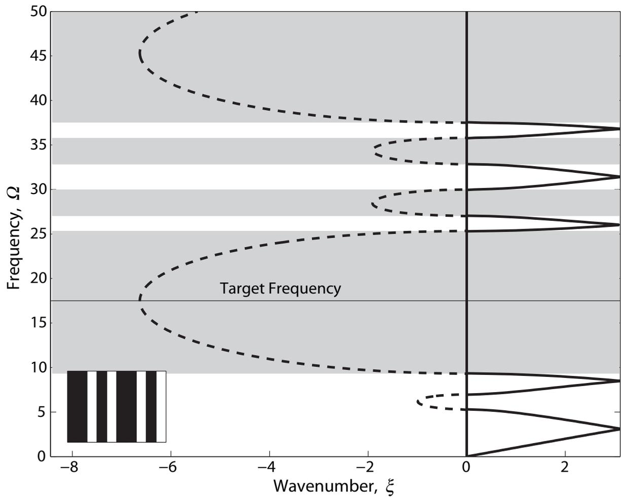
Figure 7 Frequency spectrum for unit cell design optimized for maximum attenuation at non-dimensional frequency  $\Omega^* = 17.5$ . (—) Real part (pass band), (---) Imaginary part (stop band). Stop bands are shaded. Design is shown in inset and has a binary code of '0010100101' (black: stiff material, white: compliant material).
