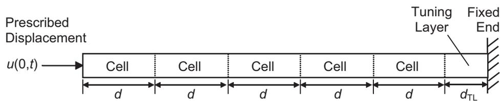
Figure 5 Schematic showing a synthesized structure composed of five cells and a tuning layer placed at the far right end. Length of tuning layer is denoted  $d_{TL}$ . The excitation is harmonic at  $\Omega^* = 20$  and is applied at the left end.
