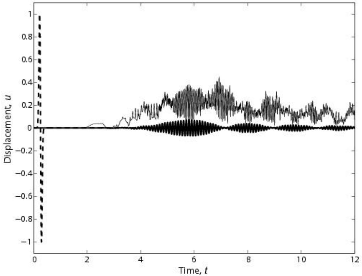
Figure 13 “Input” and “output” displacements for banded structure designed to isolate a shock pulse applied at the left end. The frequency content of the input pulse (given by Eqs. (28)-(29)) covers the range  $0 \leq \Omega^* \leq 50$ . ( - - ) Prescribed displacement at left end (input), ( — ) Displacement close to right end at position O (output), ( — ) Maximum displacement within 5th cell (which also represents the degree of transmission).
