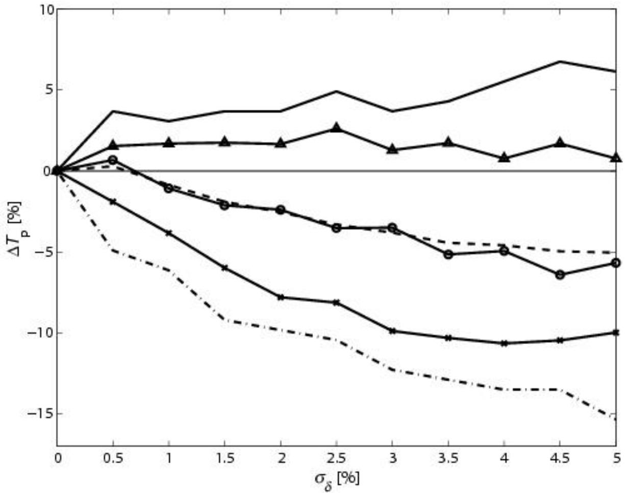
Figure 27 Sensitivity distribution quantities pertaining to the change of frequency spectrum characteristics (i.e.,  $\Delta T_p$  within  $0 \leq \Omega^* \leq 50$ ) as a result of statistical variations in layer thicknesses of unit cell ‘0010110111’ (see Fig. 11). (—) Maximum, (---) Average, (- · -) Minimum, (—▲—) 95th percentile, (—○—) 50th percentile, (—×—) 5th percentile.
