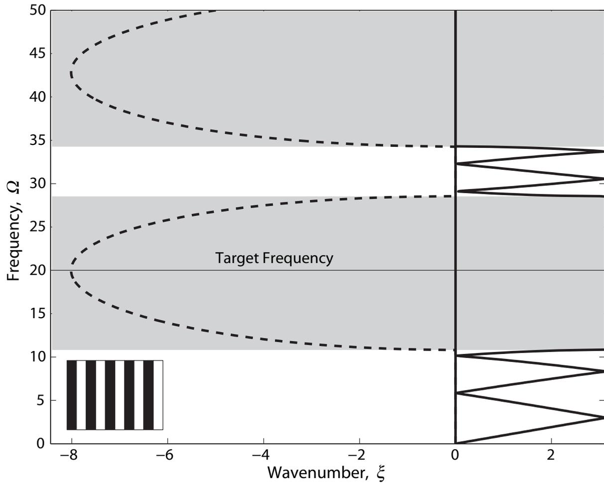
Figure 2 Frequency spectrum for optimal unit cell design for case involving harmonic excitation at non-dimensional frequency  $\Omega^* = 20$ . ( — ) Real part (pass band), ( - - ) Imaginary part (stop band). Stop bands are shaded. Design is shown in inset and has a binary code of '0101010101' (black: stiff material, white: compliant material).
