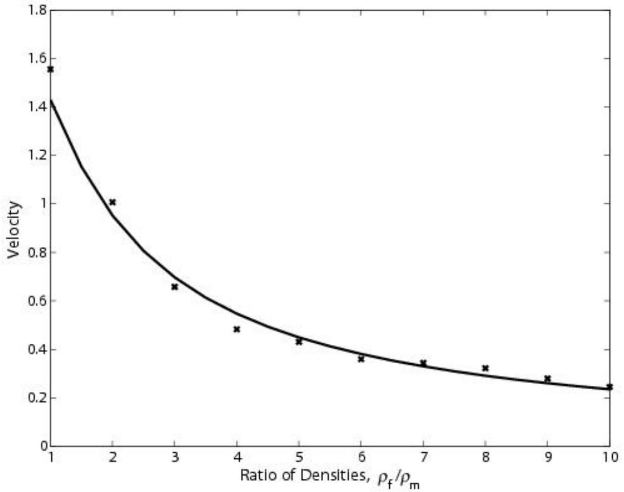
Figure 22 Velocity versus density ratio  $\rho_f/\rho_m$  for both infinite media and a finite (five) number of cells (as shown in Fig. 20). ( — ) Infinite:  $\max(c_g)$  within 2<sup>nd</sup> pass band, (X) Finite:  $\alpha$ .
