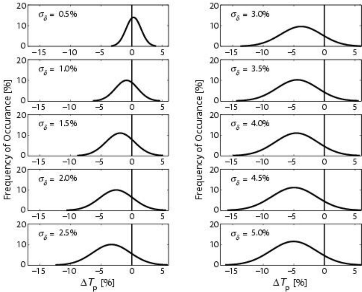
Figure 26 Sensitivity of frequency spectrum characteristics to statistical variations in layer thicknesses of unit cell ‘0010110111’ (see Fig. 11). The change of the transmissibility within frequency range of interest (i.e.,  $0 \leq \Omega^* \leq 50$ ) is denoted  $\Delta T_p$ .
