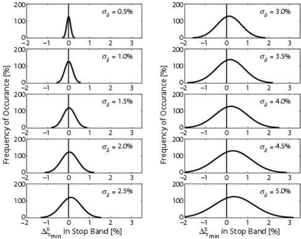
Figure 24 Sensitivity of frequency spectrum characteristics to statistical variations in layer thicknesses of unit cell ‘0101010101’ (see Fig. 2). The change of the absolute value of the imaginary wavenumber at the center of the stop band of interest (i.e., at  $\Omega^* = 20$ ) is denoted  $\Delta\xi_{\min}$ .
