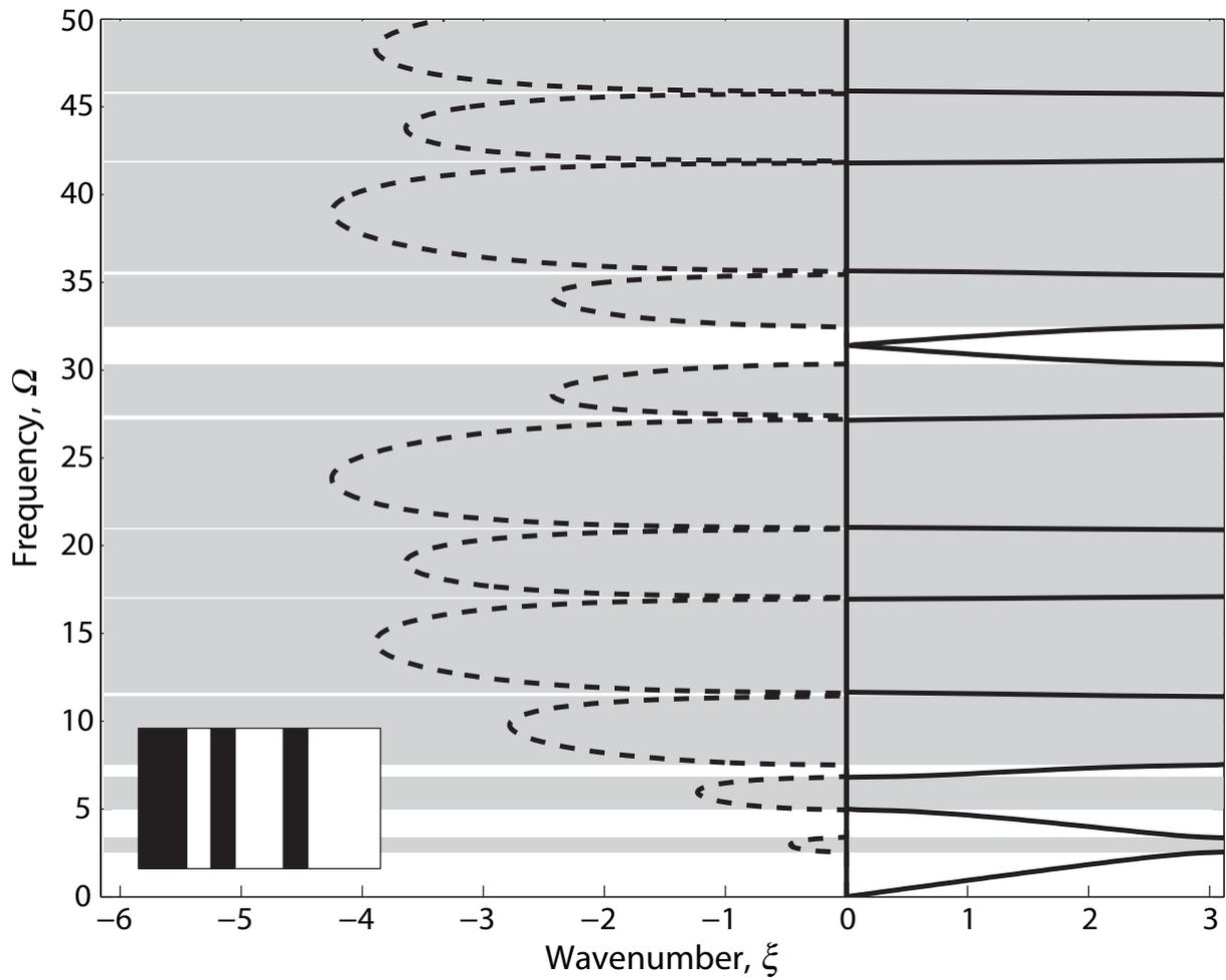
Figure 11 Frequency spectrum for optimal unit cell design for case involving general transient excitation at non-dimensional frequency range of  $0 \leq \Omega^* \leq 50$ . ( — ) Real part (pass band), ( - - ) Imaginary part (stop band). Stop bands are shaded. Design is shown in inset and has a binary code of '0010110111' (black: stiff material, white: compliant material).
