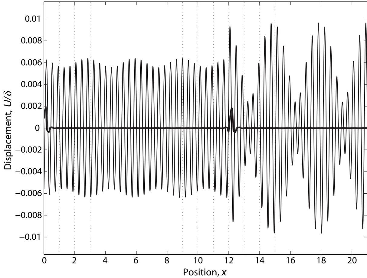
Figure 10 Spatial response of partially periodic structure shown in Fig. 8a when subjected to both excitations  $f_1$  and  $f_2$ . The response of the equivalent homogenous structure is superimposed. ( — ) Banded structure, ( — ) Homogenous structure. Vertical dotted lines indicate boundaries of designed periodic cells within structure.
