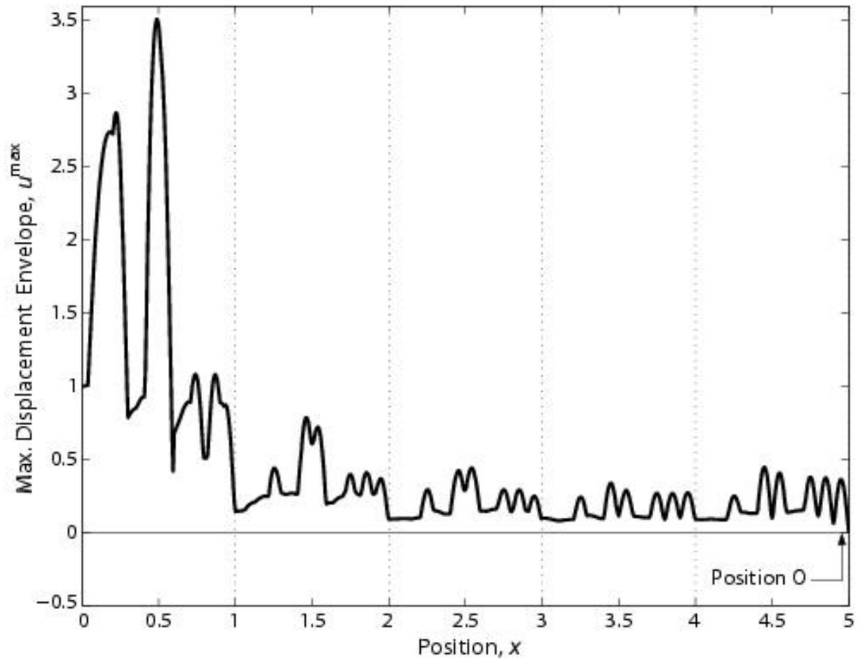
Figure 14 Envelope of maximum displacement throughout duration of numerical simulation (12 seconds) in banded structure designed for shock isolation. The shock load (given by Eqs. (28)-(29)), with frequency content spanning the range  $0 \leq \Omega^* \leq 50$ , is applied at the left end.
