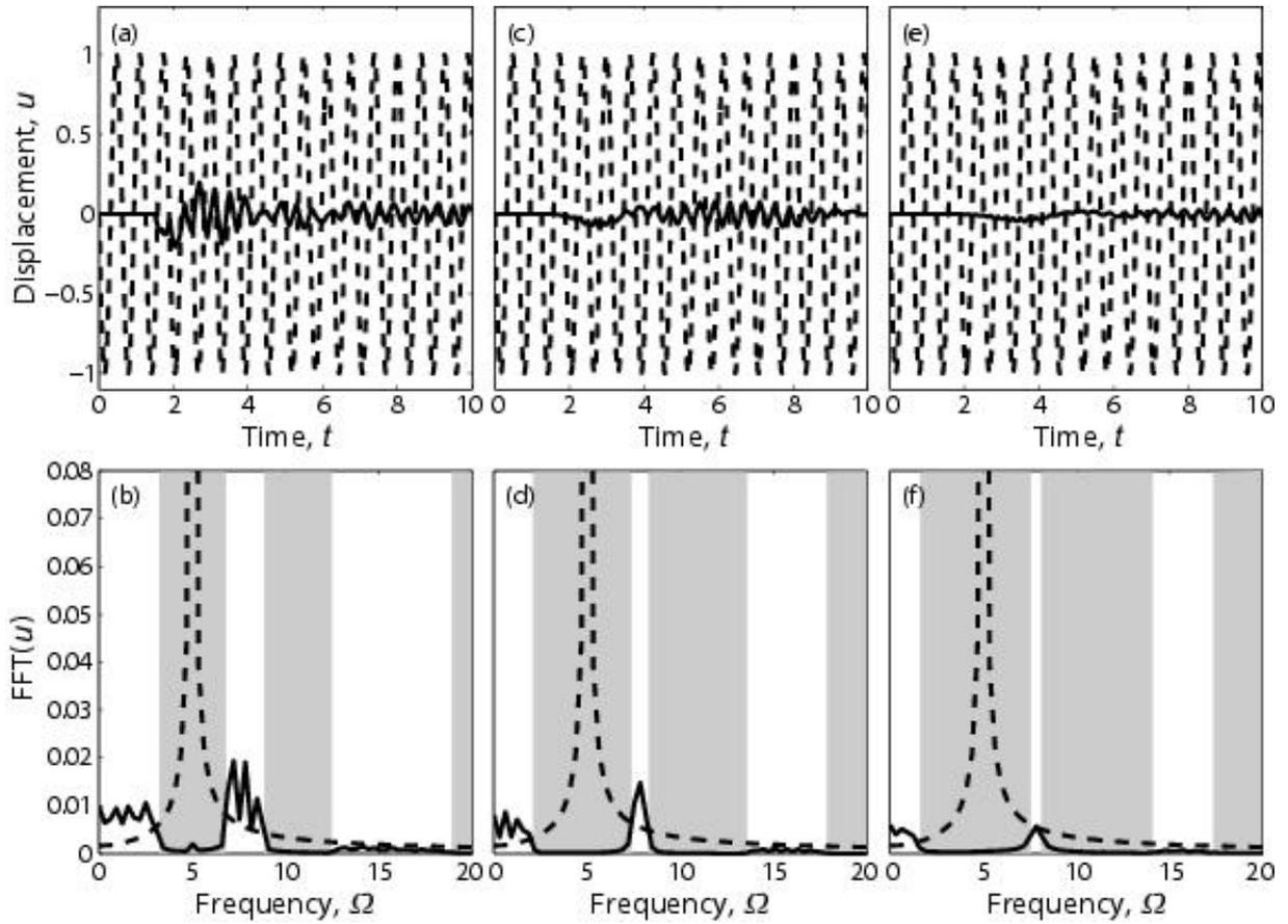
Figure 21 “Input” and “output” displacements in Fig. 20 structure for the following cases:  $\rho_f / \rho_m = 2$  in (a) time and (b) frequency domains,  $\rho_f / \rho_m = 5$  in (c) time and (d) frequency domains, and  $\rho_f / \rho_m = 9$  in (e) time and (f) frequency domains. ( - - ) Input at left end, ( — ) Output at end of 5<sup>th</sup> cell. Stop-band frequency ranges for the employed unit cell are shaded in the frequency domain plots.
