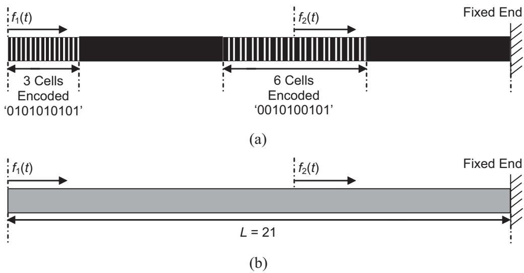
Figure 8 (a) Finite structure partially composed from cells encoded '1010101010' (Fig. 1) and '0010100101' (Fig. 7) while most of the structure is homogenous. (b) Statically equivalent homogenous structure. The length of both structures is  $L = 21$ . Excitation locations are shown.
