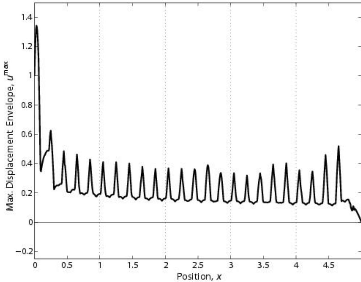
Figure 4 Envelope of maximum displacement throughout duration of numerical simulation (12 seconds) in banded structure designed for vibration isolation. The excitation is harmonic at  $\Omega^* = 20$  and is applied at the left end of the structure.
