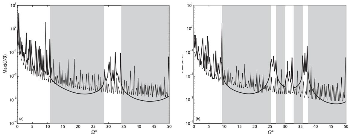
Figure 9 Frequency response of partially periodic structure shown in Fig. 8 when subjected (a) only to excitation  $f_1$ , and (b) only to excitation  $f_2$ . Stop-band frequency ranges are shaded for unit cell encoded (a) ‘1010101010’, and (b) ‘0010100101’. The response of the equivalent homogenous structure is superimposed for both cases. (—) Banded structure, (—) Homogenous structure.
