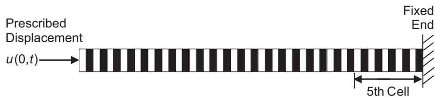
Figure 3 Banded structure designed for achieving vibration isolation. The structure is formed from the synthesized unit cell encoded '0101010101', shown in Fig. 2, with reverse order of layering to minimize displacement at the receiving end. Its length is  $L = 5$ . The excitation is harmonic at  $\Omega^* = 20$  and is applied at the left end.
