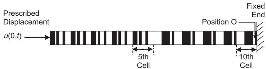
Figure 17 Banded structure designed for enhanced achievement of shock isolation over frequency range  $0 \leq \Omega^* \leq 50$ . The structure is formed from the synthesized unit cells '0010110111' (Fig. 11) and '1111000010' (Fig. 15). Five cells of the latter are stacked adjacent to five cells of the former. The structure's length is  $L = 10$ . The shock excitation  $u(0,t)$  is given by Eqs. (28)-(29).
