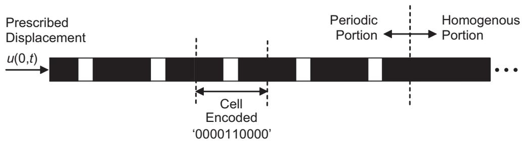
Figure 20 Structure consisting of five periodic cells of type '0000110000' and an extended homogenous portion. Loading in the form of prescribed harmonic displacement (starting at  $t = 0$ ) at  $\Omega^* = 5$  is applied at the left end.
