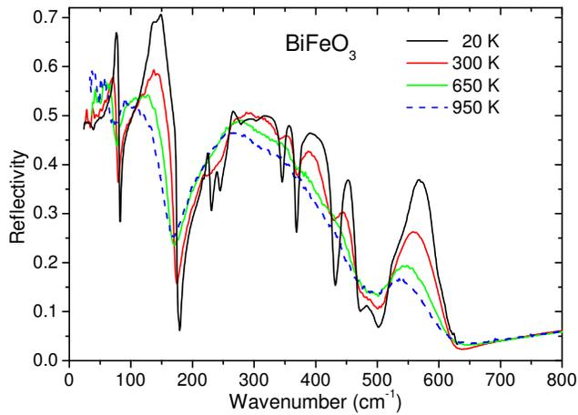
FIG. 1: (Color online) Temperature dependence of the IR reflectivity spectra of BiFeO<sub>3</sub> ceramics. We note that the reflectivity value above 200 cm<sup>-1</sup> may be slightly reduced due to a small porosity of the ceramics and subsequent diffuse scattering of the IR beam. This can apparently enhance the phonon damping in the fit of our spectra, but the phonon frequencies are not substantially influenced.
