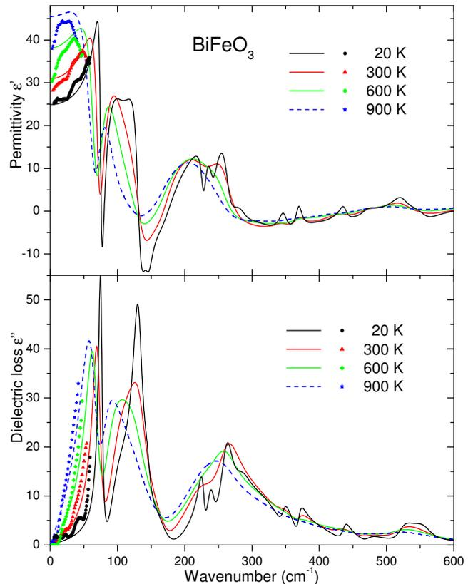
FIG. 2: (Color online) Complex dielectric spectra of BiFeO<sub>3</sub> at selected temperatures. The dots are experimental THz data, lines are results of the reflectivity fits. Note the shifts of  $\varepsilon''$  peaks to lower frequencies due to the phonon softening on heating.
