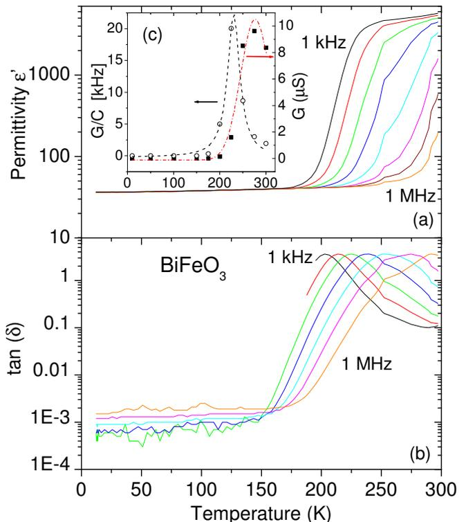
FIG. 4: (Color online) Temperature dependence of the low-frequency permittivity (a) and dielectric loss (b) in BiFeO<sub>3</sub> ceramics. Low-frequency  $\tan \delta$  is not shown at low temperatures due to the high noise. Inset (c) shows the temperature dependence of conductance  $G$  (full symbols) and ratio of conductance and capacitance  $G/C$  (empty symbols).
