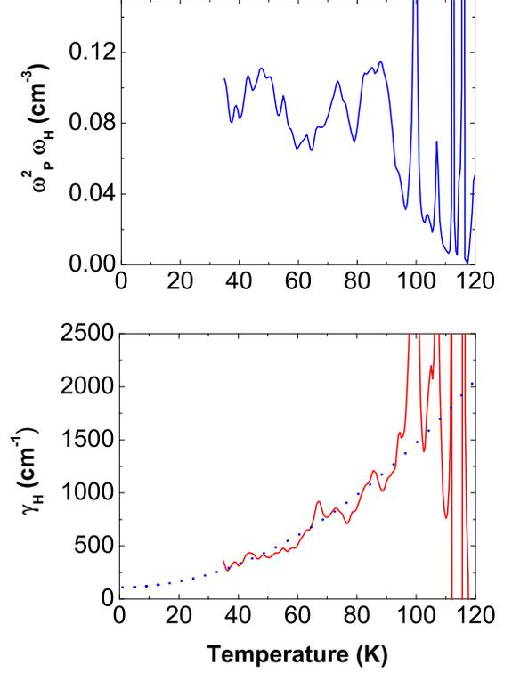
FIG. 3: Drude carrier analysis of the low-T  $\Delta\sigma_{xy}$ . (a) Squared plasma frequency  $\omega_p^2(T)$  times Hall frequency  $\omega_H(T)$  (b) Hall scattering rate  $\gamma_H(T)$ . Dashed line shows a fit with  $\gamma_H(T)=\gamma_0 + aT^2$ .
