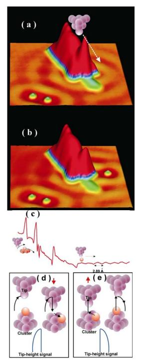
**Figure 1.** Atom extraction. (a) A three-dimensional STM image of a silver nanocluster deposited by tip-surface contact. The tip is brought close to the protruded part of the cluster and then moved laterally towards a destination on the Ag(111) surface. (b) An STM image acquired after this procedure shows a height reduction of the cluster protrusion and the extracted atom at the final surface destination. (c) The manipulation signal of this event reveals the atomistic
