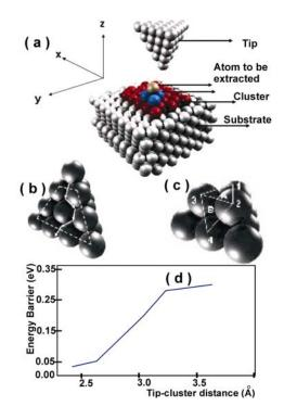
**Figure 4.** Theoretical modeling of the tip-cluster junction. (a) The geometry of the tip, adatom, cluster and silver substrate used for the calculation. (b) The minimum energy diffusion path of the atom after extraction with the STM-tip. (c) Transferring of the atom from A to B, and from B to A will cost the same energy. (d) The energy barrier to extract the top-most atom in the cluster as a function of the tip-cluster distance.
