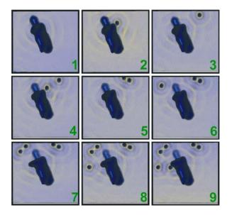
**Figure 2.** Atom-by-atom extraction sequence. A sequence of STM images from an STM movie [23] shows atom-by-atom extraction from a silver cluster. This series proves the reliability of our atom extraction process.
