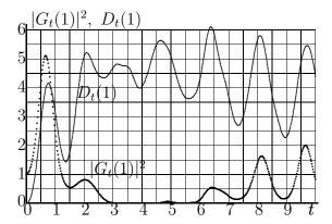
FIG. 1. Amplification coefficient  $g = G_t^2$  and noise  $D_t$  versus t at x = 1 for the Cummings-Tavis amplifier with N = 10 atoms. At t = 0,  $G^2 = 1$  (thick dotted line) and D = 0 (thin line).
