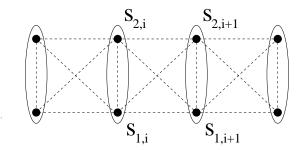
FIG. 1. A generalized spin $\frac{1}{2}$  ladder with all possible isotropic exchange interactions between nearest-neighbor rungs. O vals show spin pairs whose states are involved in the elementary matrix  $g_i$  de ned by (3). Couplings are described in the text, see (4).
