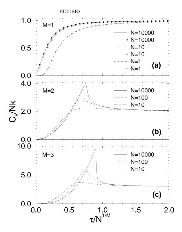
FIG. 1. The specific heat of a finite number N of bosons confined in an isotropic parabolic potential as a function of the dimensionless temperature  $\tau/N^{1/M} = kT/(\hbar\omega N^{1/M})$ , where M is the spatial dimension for (a) M = 1, (b) M = 2, and (c) M = 3. The lines are results of the iterative scheme for different values of N. The symbols in (a) are the results obtained using the exact expression Eq.(12).
