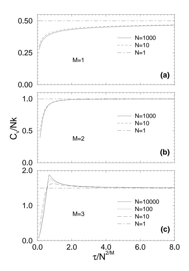
FIG. 4. The specific heat of N bosons confined in M-dimensional rigid box as a function of the dimensionless temperature  $\tau/N^{2/M} = 8mkTL^2/h^2N^{2/M}$  for (a) M = 1, (b) M = 2, and (c) M = 3. Results are obtained using Eqs.(20)-(22) within the integral approximation.
