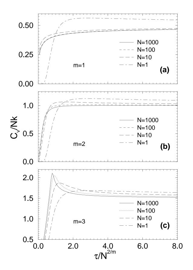
FIG. 3. The specific heat of N bosons confined in M-dimensional rigid box as a function of the dimensionless temperature  $\tau/N^{2/M} = 8mkTL^2/h^2N^{2/M}$  for (a) M = 1, (b) M = 2, and (c) M = 3. Results are obtained using Eqs.(15)-(17) by summing up the infinite series for  $\Theta_j(b)$  to convergence.
