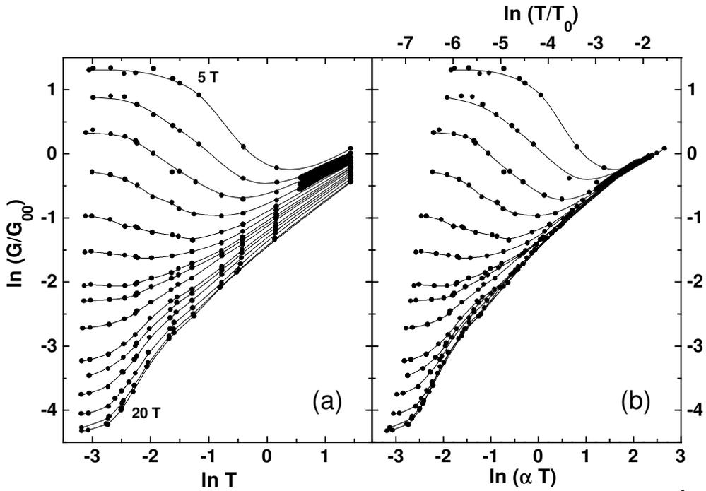
FIG. 3. Conductance per single  $\text{CuO}_2$  plane,  $G$ , normalized to  $G_{00} = e^2/2h$  for InS1 in magnetic fields ranging from 5 T (topmost curve) to 20 T (lowest curve), plotted (a) versus temperature on a logarithmic scale, and (b) versus temperature scaled by the factor  $(B)$ , or, equivalently (upper scale), by  $T_0(B)$ .
