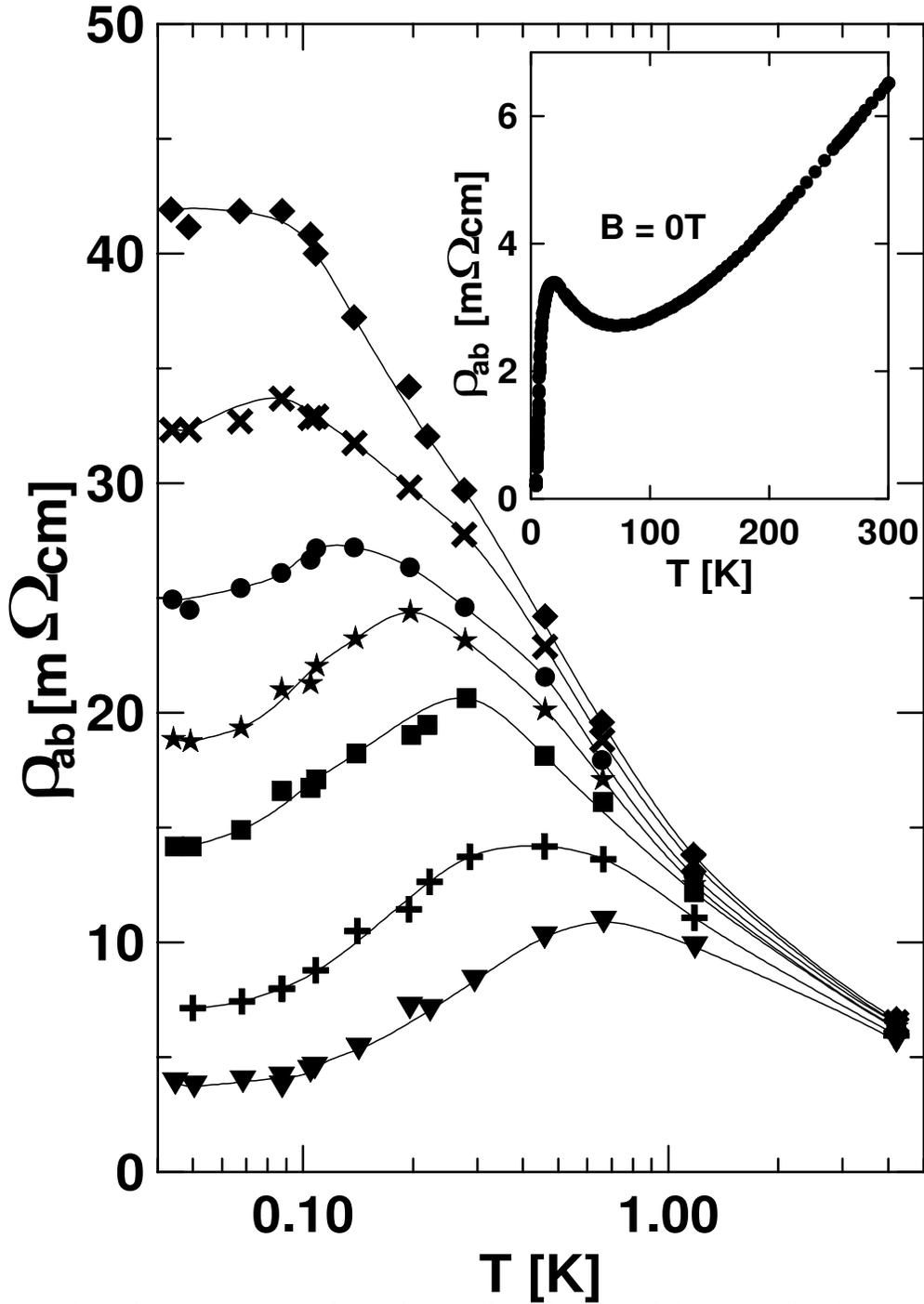
FIG .1. The temperature dependence of  $\rho_{ab}$  for InS1 in perpendicular magnetic fields. The fields are, from below, 7, 8, 9, 9.4, 9.8, 10.2, 10.6 T. The open circles between  $T = 0.7$  K and  $T = 1$  K show the data obtained with dc as explained in the text. The lines are guides to the eye. The inset shows  $\rho_{ab}(T)$  in zero field.
