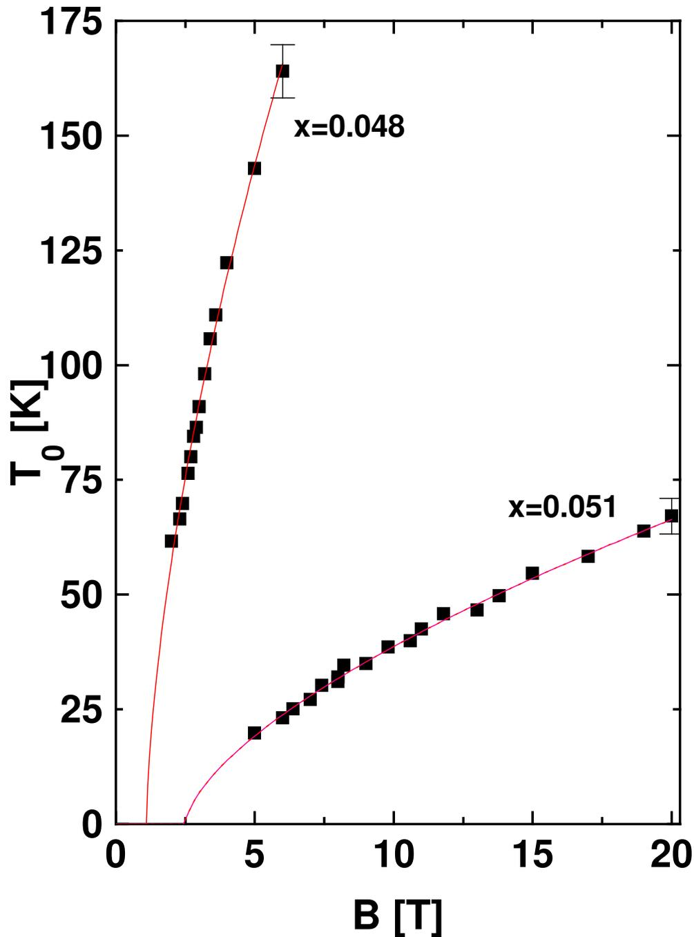
FIG. 5. The dependence of the parameter  $T_0$  on magnetic field for samples S1 ( $x = 0.051$ ) and S2 ( $x = 0.048$ ). The error bars show the uncertainty resulting from the fit of the Motz relation to the data for the highest magnetic field. The dashed lines show the expression  $T_0 = A [(B - B_{cr}) / B_{cr}]^n$ , fitted to the data, with the parameters  $A$ ,  $B_{cr}$ , and  $n$ , as described in the text.
