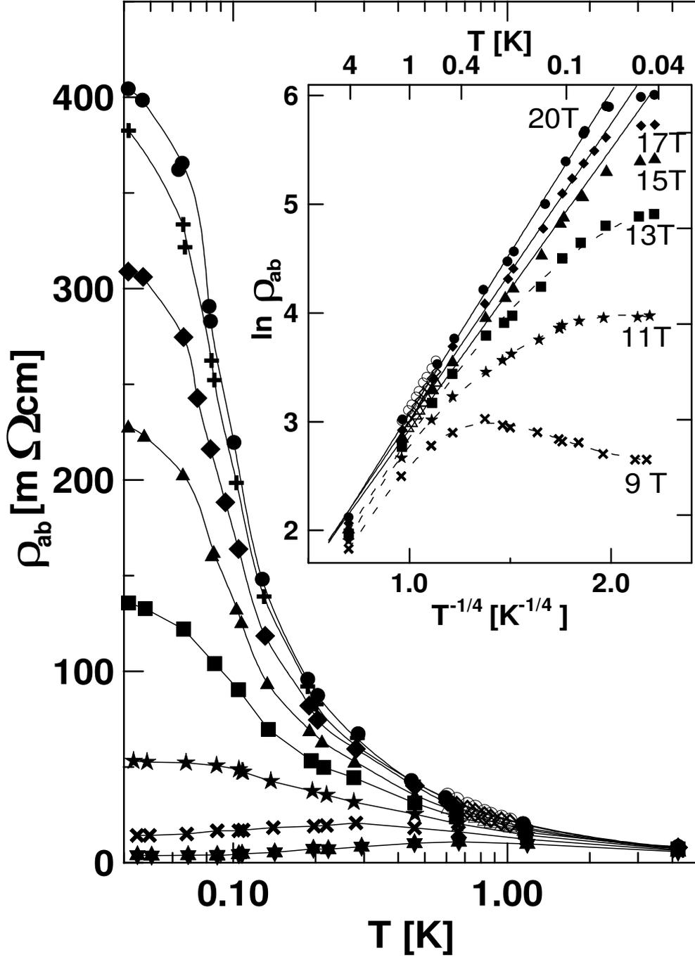
FIG. 2. The temperature dependence of  $\rho_{ab}$  for InSb in perpendicular magnetic fields. The fields are, from below, 7, 9, 11, 13, 15, 17, 19, and 20 T. The open circles between  $T = 0.7$  K and  $T = 1$  K show the data obtained with dc as explained in the text. The lines are guides to the eye. The inset shows  $\ln \rho_{ab}$  versus  $T^{-1/4}$  for several magnetic fields.
