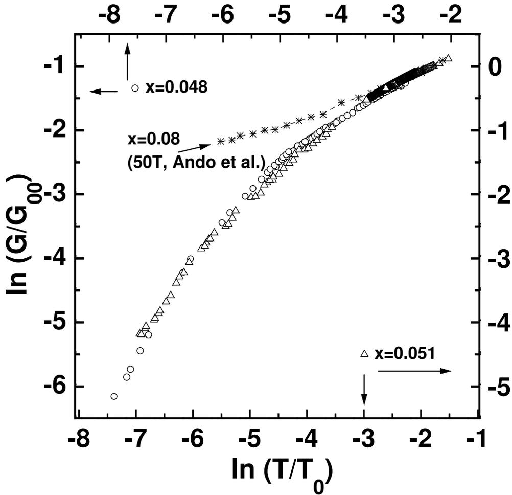
FIG. 4. Log-log graph of the scaled normal state conductance as a function of the scaled temperature for samples S1 and S2, and for the single crystal from Ref. [4].
