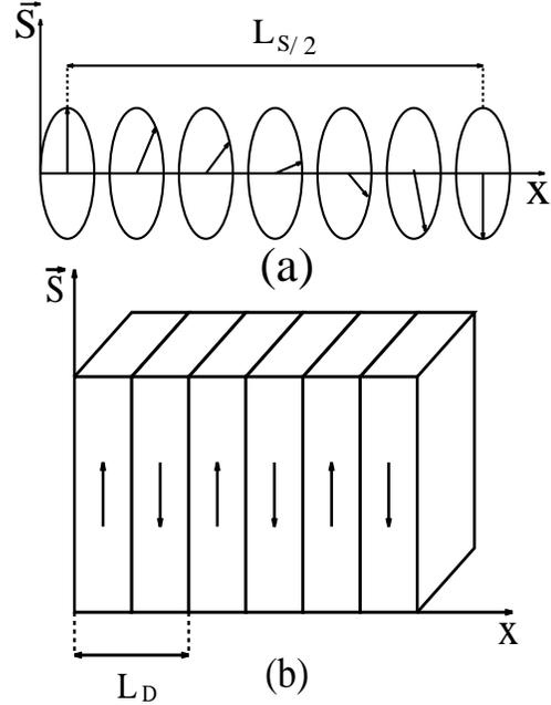
FIG. 1. (a) The spiral magnetic structure  $S(x)$ , with the period  $L_S$  in the superconducting phase for small anisotropy  $D = \chi_{ex} < 10^3$ . (b) The domain-like magnetic structure  $S(x)$ , with the period  $L_D$  in the superconducting phase for appreciable anisotropy  $D = \chi_{ex} > 10^3$ .
