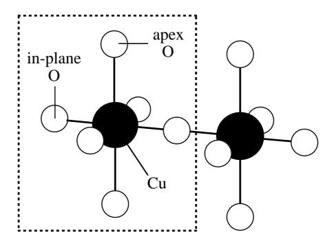
Figure 1. The cluster model  $\text{Cu}_2\text{O}_{11}$ .
