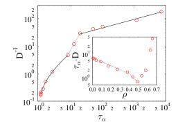
FIG. 4. The diffusivity, D, as a function of the  $\alpha$ -relaxation time,  $\tau_{\alpha}$ . As in real experiments three different regions appear. The superimposed curves are fit with the generalized fractional Stokes-Einstein law  $D^{-1} \sim \tau_{\alpha}^{\xi}$ . Inset: The product of diffusivity,  $D(\rho)$ , and of  $\alpha$ -relaxation time,  $\tau_{\alpha}(\rho)$ , as a function of density  $\rho$ .
