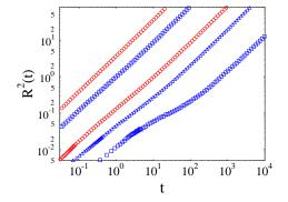
FIG. 3. Particles mean square displacement,  $R(t)^2$ , as a function of time in a system of linear size L = 16, for J = 10, and for  $\rho = 0.088, 0.271, 0.440, 0.581, 0.674$  (higher curves correspond to lower densities).
