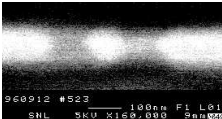
Figure 4: Scanning electron micrograph of a SET-like geometry sample, made by shadow evaporation, before anodisation.
