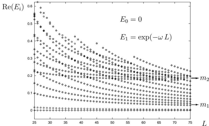
**Figure 2.** Dependence of the spectrum on system size. The data is from numerical diagonalization for  $a = \frac{1}{4}$ ,  $h = 0.3$ . Shown are the real parts of the eigenvalues of  $H$ . The gaps  $m_1$  and  $m_2$  extrapolate to finite values as seen in figure 3.
