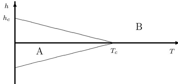
**Figure 1.** Simplified phase diagram of the three-state model. In the “low-temperature” regime A the symmetry is spontaneously broken for  $h = 0$  where  $h$  is the strength of a symmetry breaking field. It is separated by a line of spinodal points from the “high-temperature” regime B.
