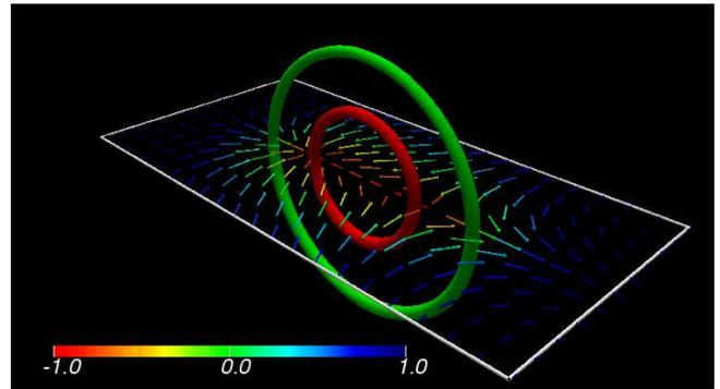
FIG. 2. The configuration of the magnetic vortex ring with  $H = 0$ ,  $p = 5.0$ , and  $a = 0$ . The vectors represent the projection of  $n$  onto the  $xy$ -plane; their colours indicate the value of  $n_z$  (refer to the colour-legend). The tubular curves illustrate the lines along which  $n = \hat{z}$  (red) and  $n = +\hat{x}$  (green). (For clarity, only the central section of the full lattice is illustrated, with a fraction of the lattice points reproduced.)
