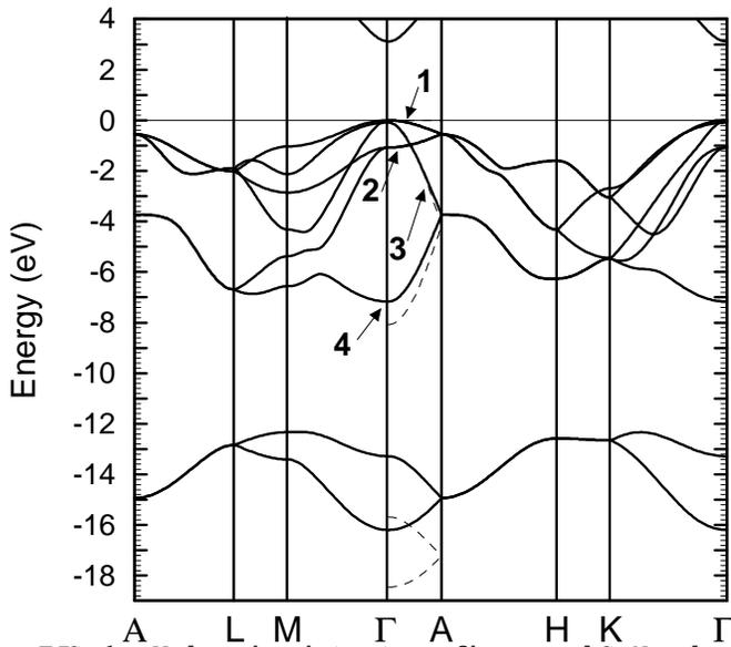
FIG. 1. Valence band structure of hexagonal GaN calculated with EHT-parameters according to Table I (solid line: set A, dashed line: set B).
