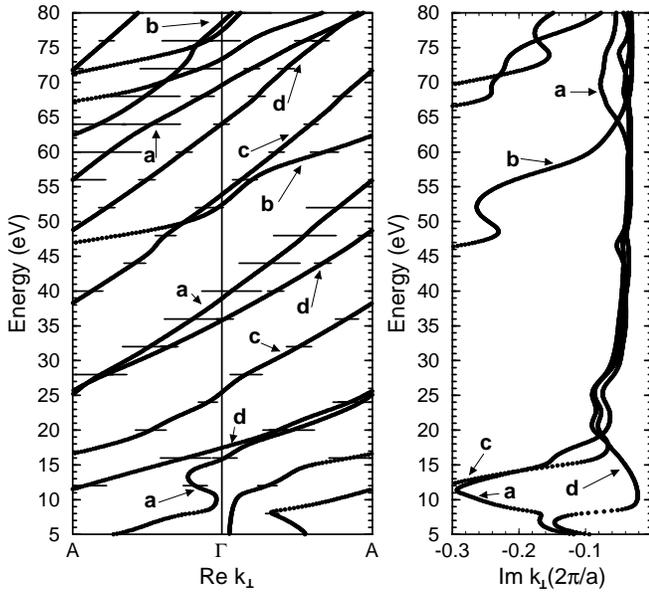
FIG. 5. Complex band structure of GaN for the symmetry line  $\Gamma$ . Bars indicate the magnitude of the expansion coefficients of the valence state with respect to the complex bulk bands.
