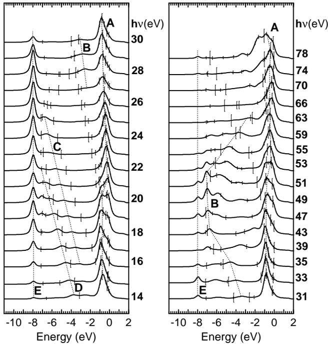
FIG. 6. Theoretical normal emission spectra for GaN (0001)-(1x1)Ga. We have normalized each spectrum separately to an equal amount in the maximum of the photocurrent. The bars indicate binding energies at which direct transitions would be positioned. Their dispersion is drawn by dotted lines as a guide the eye. The energy zero is the VBM, the light is chosen incident along the xz plane with p-polarisation. The spectra are calculated from set A in Table (I).
