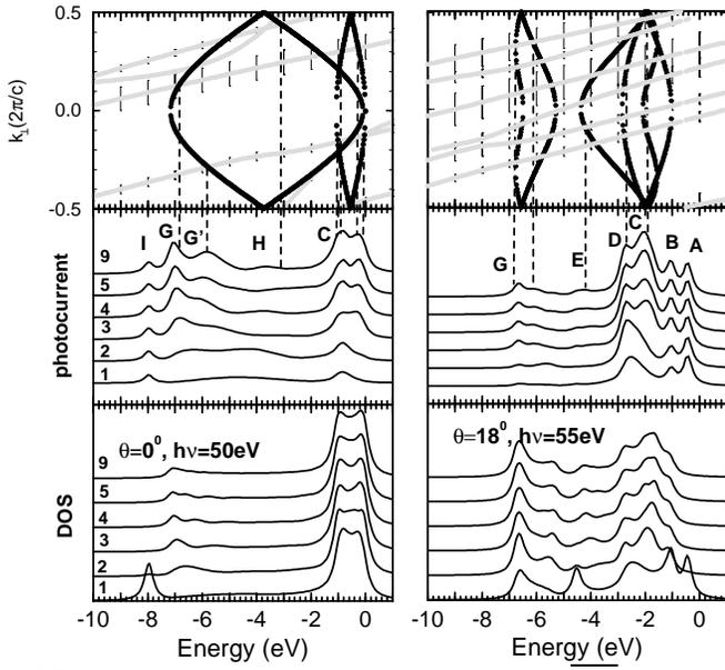
FIG. 9. Layer resolved photocurrent in the M direction for 0 and 18 (middle part) together with the complex bands (grey) and the initial bulk bands (dots) in the top panel. The bands are shifted by the excitation energy and the positions of direct transitions are indicated (vertical dashed lines). The bottom panel shows the layer-resolved density of states. The layer resolved photocurrent is calculated for the number of layers as indicated, each layer consisting of four atomic planes (see text).
