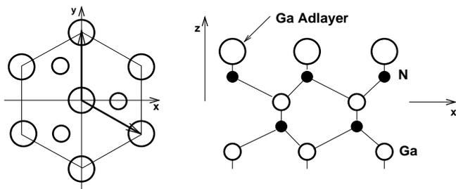
FIG. 2. The geometry of the GaN (0001)-(1x1) Ga surface according to [5].
