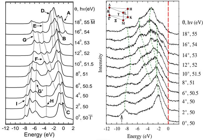
FIG. 10. Results for the M direction. On the left hand side the theoretical photocurrents according to parameter set A, and on the right hand side experimental data from Dhesi et al. [8]. The arrow indicates a weak shoulder to be compared with (I) (see text)
