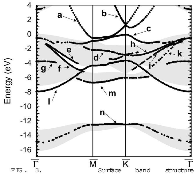
FIG. 3. Surface band structure of the GaN (0001)-(1x1) Ga surface and the projected GaN bulk band structure (shaded). For the calculation parameter set A according to Vogel et al. [2] was used.
