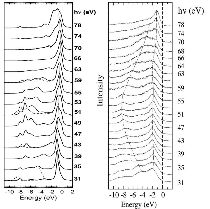
FIG. 8. Comparison between theoretical (left hand side) and experimental photoemission spectra of Desiet al. [8] in normal emission. The theoretical spectra are calculated from set A (see Table I), except for the dashed spectra, which are calculated from set B.
