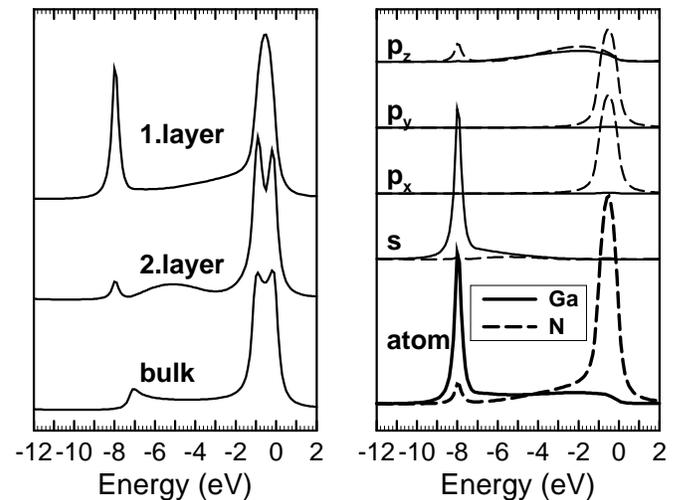
FIG. 4. Density of states at  $\bar{\Gamma}$  for GaN (0001)-(1x1) Ga. On the left hand side the layer resolved DOS is shown, while on the right the DOS of the first layer is further resolved into its atomic and orbital contributions. Calculated with the parameters from set A (see Table I).
