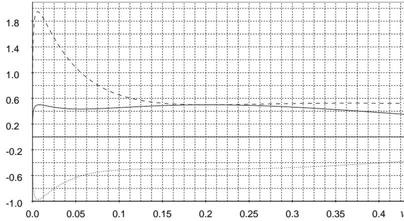
**Fig. 12:** The evolution of  $\hat{f}^{(\sigma\sigma)}$  (dashed line),  $\hat{f}^{(\sigma\tau)}$  (dotted line) and  $\hat{f}^{(\tau\tau)}$  (solid line) along the critical trajectory for the LDPC( $n, x^2, x^5$ ) ensemble.
