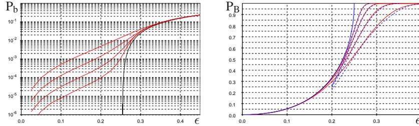
**Fig. 10:** The bit and block erasure probability for  $ELDPC(n, \lambda(x) = x, r = \frac{1}{2}, s = 1)$  for  $n = 2^i$ ,  $i = 8, 10, 12, 14$ . As can be seen from the picture, the block erasure curves actually converge to a limiting (non-zero) curve over the whole range of  $\epsilon$ , whereas the bit erasure curves decrease to zero below the threshold for increasing block lengths. Also shown are the result of using the scaling laws for the block erasure probability as stated in Lemma 3.2.
