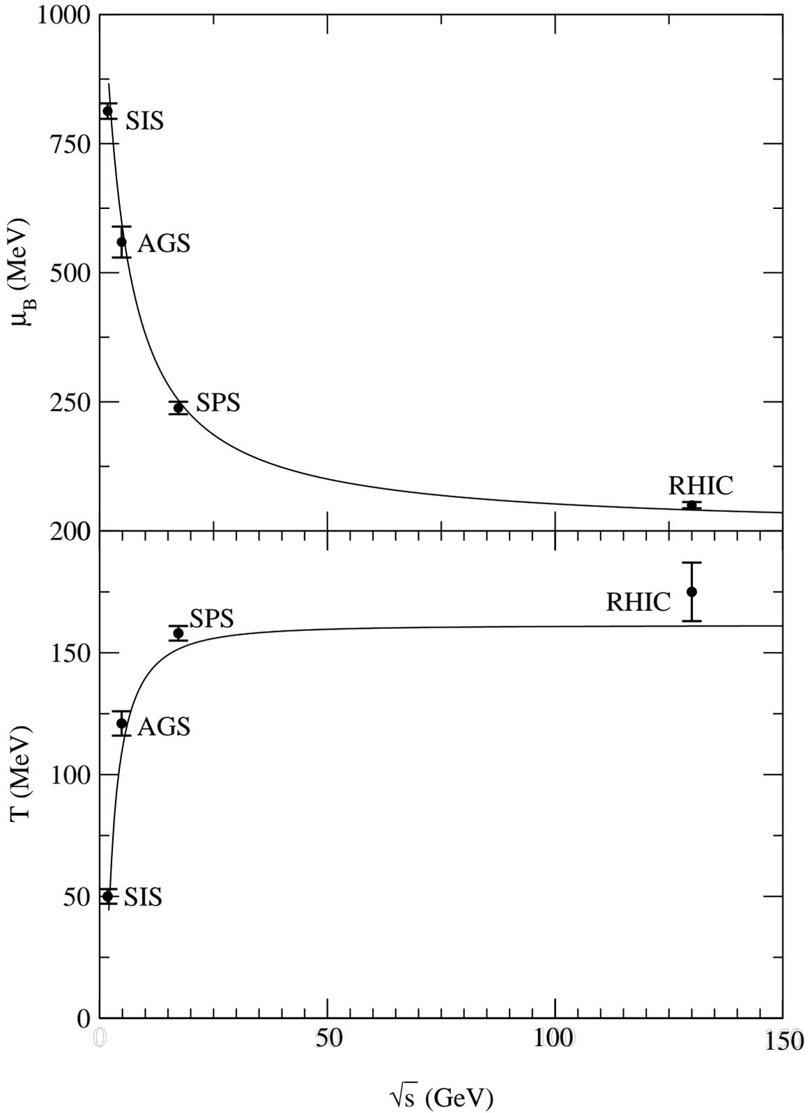
Figure 1: Behavior of the freeze-out baryon chemical potential  $\mu_B$  (upper curve) and the temperature  $T$  (lower curve) as a function of energy. The temperature  $T$  as a function of beam energy is determined from the unified freezeout condition  $\mu_B = \mu_N = 1$  GeV [13].
