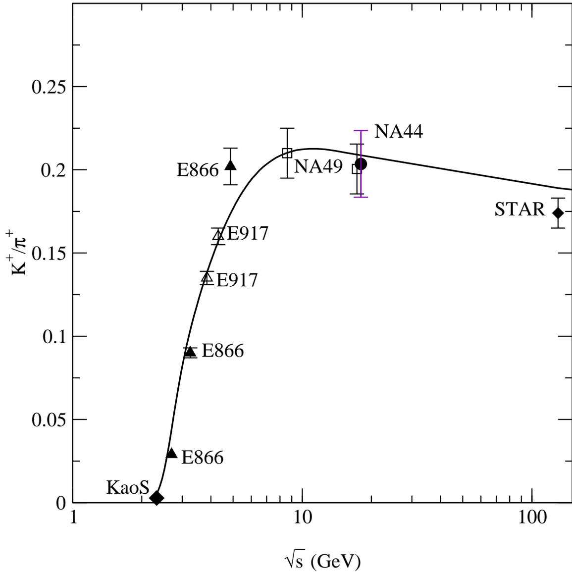
Figure 5:  $K^+/\pi^+$  ratio obtained around midrapidity as a function of  $\sqrt{s}$  from the various experiments. For the references for all data points see [3, 6]. The full line shows the results of the statistical model in complete equilibrium. The value at RHIC was estimated using results from the STAR collaboration on the  $K^-/\pi^-$  and  $K^+/\pi^+$  ratios, assuming  $K^-/\pi^- = K^+/\pi^+ = 1.007$ .
