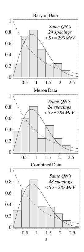
FIG. 2: Histograms of the nearest-neighbor mass spacing distribution for hadron states with same QNs. Curves represent the Poisson (dashed) and Wigner (solid) distributions.
