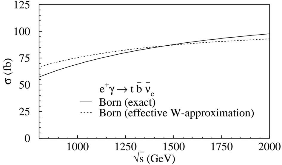
Figure 5.4: Total cross section for the process  $e^+ \gamma \rightarrow t \bar{b} \bar{\nu}_e$ . The full line shows the exact result while the dashed line shows the result using the effective  $W$ -approximation.
