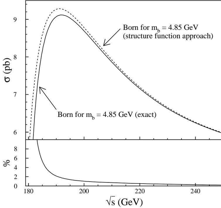
Figure 5.3: Total born cross section for the process  $W^+ \gamma \rightarrow t \bar{b}$  for unpolarized W-Bosons. The upper figure compares the structure function approach with the fixed order calculation for massive  $b$ -quarks. The lower figure shows the deviation of the structure function approach from the massive calculation in percent.
