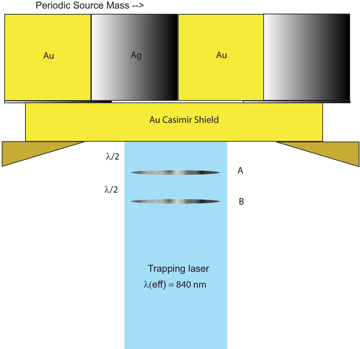
FIG. 3: Proposed experimental arrangement. The standing wave cavity formed by reflection from the Au Casimir shield is used to trap BEC atoms in the two potential wells nearest to the periodic source mass array.
