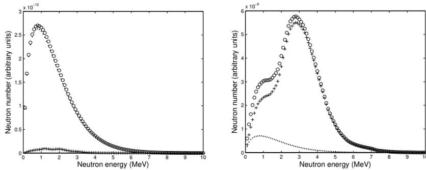
Fig. 1. Simulated neutron energy spectra for the dewar (left) and LEM (right). The dotted line is the contribution from spontaneous fission, the crossed line the contribution from  $(\alpha, n)$  reactions and the circled line is the sum of the two.
