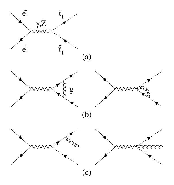
Figure 1: Generic diagrams for  $\tilde{t}_1 \bar{\tilde{t}}_1$  production in  $e^+e^-$  collisions. (a) Born level; (b) virtual QCD corrections; (c) gluon radiation.
