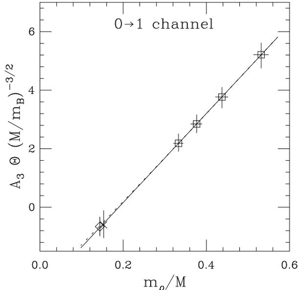
**Figure 4**  $1/M$  extrapolation for  $A_3$  for the  $0 \rightarrow 1$  channel, from the charm scale to the bottom scale. The squares are measured points for our four heavy mass values, which are extrapolated linearly (solid curve) or quadratically (dashed curve) in  $1/M$  to the  $B$  scale (diamond or cross). The extrapolated points have been displaced slightly for clarity.
