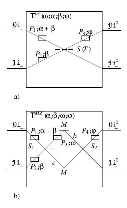
FIG. 1: A universal quantum interference device operating on a qubit can be realized by a 4-port interferometer with two input ports  $\mathfrak{Di}$ ;  $\mathfrak{Ji}$  and two output ports  $\mathfrak{Di}^0$ ;  $\mathfrak{Ji}^0$ ; a) realization by a single beam splitter S(T) with variable transmission T and three phase shifters  $P_1$ ;  $P_2$ ;  $P_3$ ; b) realization by two 50:50 beam splitters  $S_1$  and  $S_2$  and four phase shifters  $P_1$ ;  $P_2$ ;  $P_3$ ;  $P_4$ .
