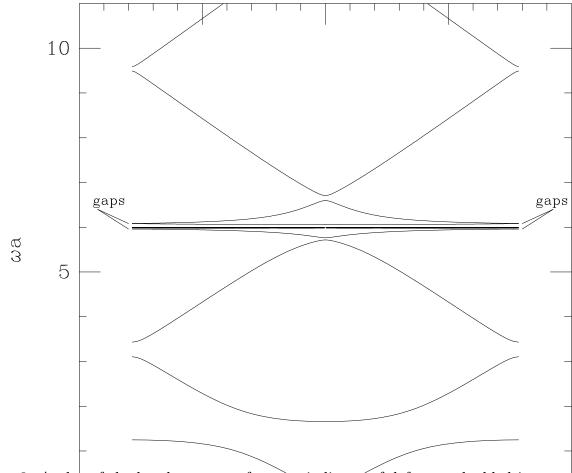
Figure 3: A plot of the band structure for a periodic set of defects embedded in a material governed by the dispersion relation in (7.7). For the defects we have again taken  $\omega_d^2 a^2 = 2,44\pi N_d \omega_d^2 \Delta^2 a^3 \equiv 4$ . For the parameters of the medium, we have taken  $\omega_m a = 6$  and  $32\pi N_m \rho_m \Delta^2 \omega_m^2 a^4 = 100$ . The gaps that are too small to be seen have been explicitly marked out.
