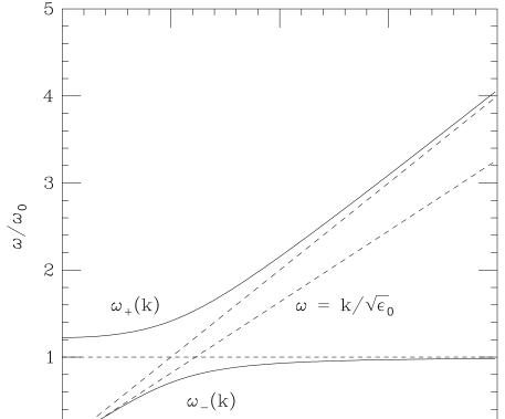
Figure 2: A plot of the dispersion relation for polaritons. Both w and k are plotted in units of  $\omega_0$ . For this plot, we have taken  $16\pi N \rho \Delta^2 \omega_0^{-2} = 1.3$  $k/\omega_0$
