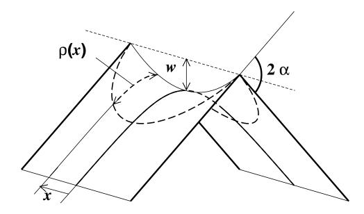
F igure 1. A minimal ridge. The boundary conditions are given by a frame (the thick solid lines) bent through an angle. The sheet is essentially at outside the region bounded by the two dashed curves, and the bulk of the energy is concentrated in this region.
