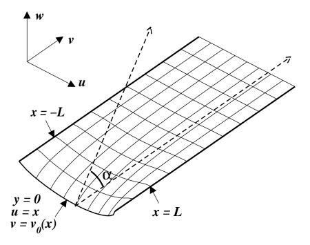
Figure 2. A schematic representation of our coordinate system and the boundary conditions imposed on the sheet. The grid is given by the lines x = constant and y = constant. The two dashed lines are the tangent to the curve x = 0 and the line  $w = w_0 (0); u = 0$  respectively, and the angle between theses lines is
