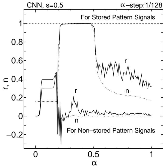
Figure 2: Correlation coefficient  $r$  (solid line) and discrimination efficiency  $n$  (dotted line) as a function of refractory parameter  $\alpha$  in CNN simulations with Eq.(2). The results for the input signals of stored and non-stored pattern trains are shown.
