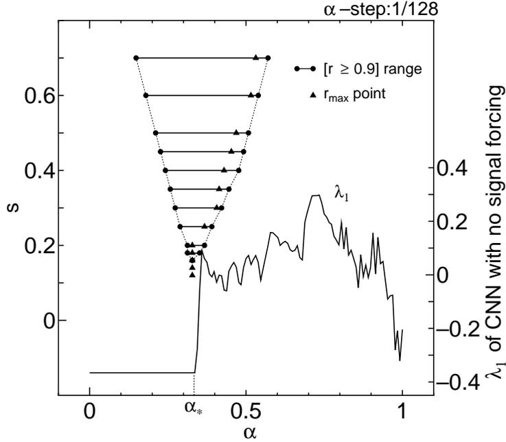
Figure 4: Dependence of the coherent  $r$ -range ( $r \geq 0.9$ ) and the  $r_{\max}$  point on the input signal strength  $s$  (the left-axis) in CNN, shown together with the maximum Lyapunov exponent  $\lambda_1$  (the right-axis) as a function of parameter  $\alpha$  in CNN with no signal forcing ( $s = 0$ ).
