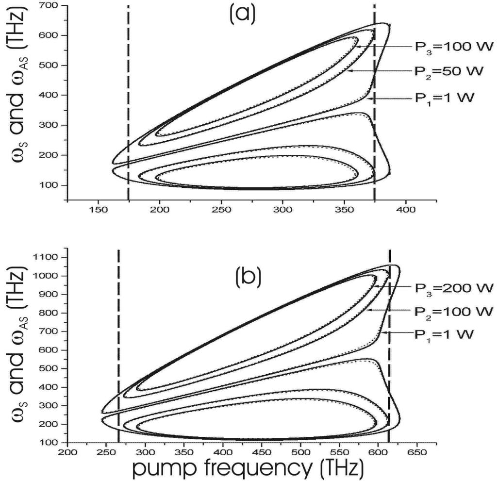
Figure 3: Diagrams showing positions of the maximal instability gain vs pump frequency calculated from Eq. (7) for different powers  $P = |E_0|^2$  in PCF (a) and TF (b). Dots show the same values calculated using phase matching condition (8). ZD points are indicated by dashed vertical lines.
