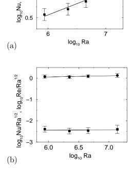
FIG. 1. (a) Nu (squares, lower curve) and Re (circles, upper curve) as a function of Ra from our simulation. The error bars are based on the variances of measured quantities which have been obtained by splitting the total time series in smaller pieces. Note that in this way we could also check that our simulations are statistically stationary. The straight lines are linear regressions giving  $Nu \sim Ra^{0.51\pm0.06}$  and  $Re \sim Ra^{0.55\pm0.02}$ .
