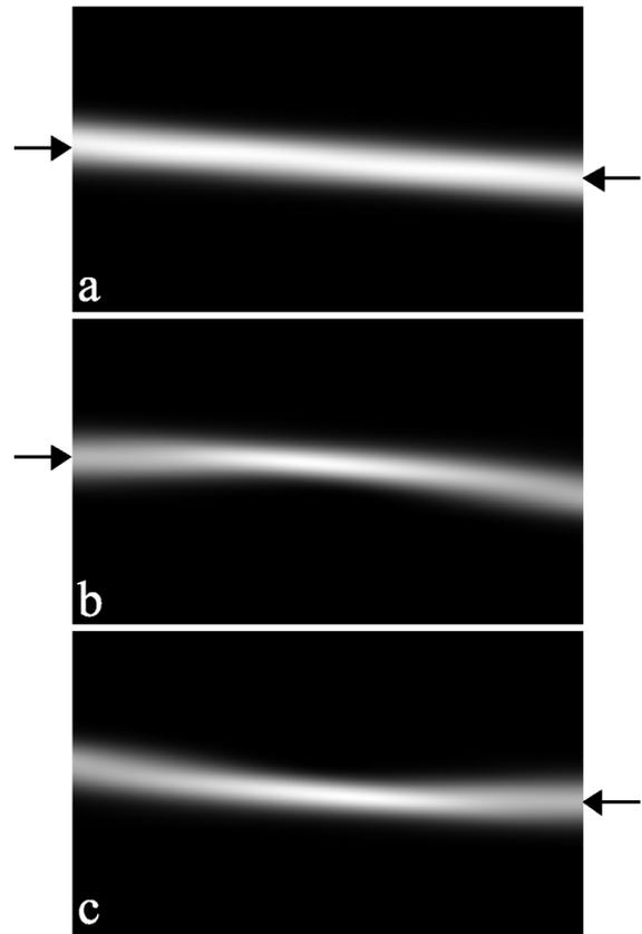
FIG. 2: Bidirectional waveguide. (a) Total intensity distribution; (b) right- and (c) left-propagating beams. Layout as in Fig. 1, parameters  $\varepsilon = 1$ , and  $\Gamma = 5$ . Initial peak intensities  $I_F = I_B = 1$ .
