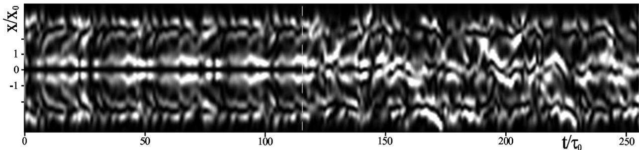
FIG. 5: Temporal evolution of the output intensity distribution of the two-lobe left-propagating beam at the left face of the crystal. Dashed line at  $t = 116\tau_0$  shows the slice corresponding to Fig. 4 (c), where the modulational instability breaks the transverse symmetry.
