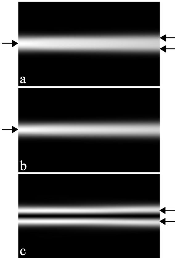
FIG. 1: Counterpropagating dipole-mode vector soliton (a), made out of a fundamental beam propagating to the right (b), and a coherent dipole beam propagating to the left (c). Coupling strength  $\Gamma = 10/3$ .
