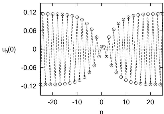
FIG. 12: Small amplitude bond-centered dark breather for an even potential with  $K_4 = -1$  and a frequency  $\omega_b = 1.99$ . The circles represent an exact solution computed numerically, having the symmetry  $u_n(t) = u_{-n+1}(t)$ . The dashed line corresponds to the analytical approximation (26).
