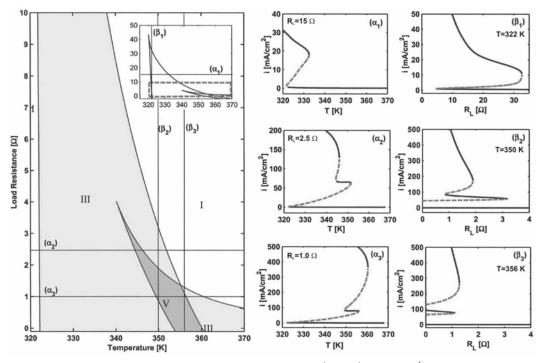
Figure 3: Two-parameter bifurcation diagram in *T* and  $R_L$  for  $n_{H2}^{in} = n_{O2}^{in} = 5.7 \times 10^{-6}$  mol/s. Regions of one, three, and five steady states are marked by I, III, and V. Corresponding one-parameter continuation diagrams with respect to temperature and to load resistance are shown in  $(\alpha_l)$ - $(\alpha_3)$  and  $(\beta_l)$ - $(\beta_3)$ respectively. The solid (dashed) curves denote stable (unstable) steady states.
