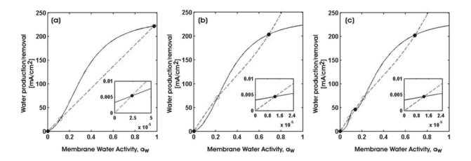
Figure 2: Water management and steady state multiplicity in a PEM fuel cell. Water production (solid curve) and removal (dashed curve) are illustrated as functions of the membrane water activity a<sub>w</sub>. The filled (empty) circles denote stable (unstable) steady states.
