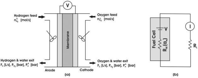
Figure 1: PEM fuel cell model
