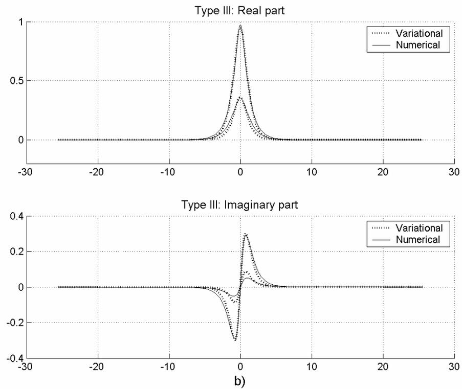
Fig. 6. Typical examples of asymmetric solitons, as found by means of the variational approximation (dashed) and in the numerical form (solid) for  $\omega = 0$  and  $\lambda = 0.2$ : (a) type I; (b) type III.
