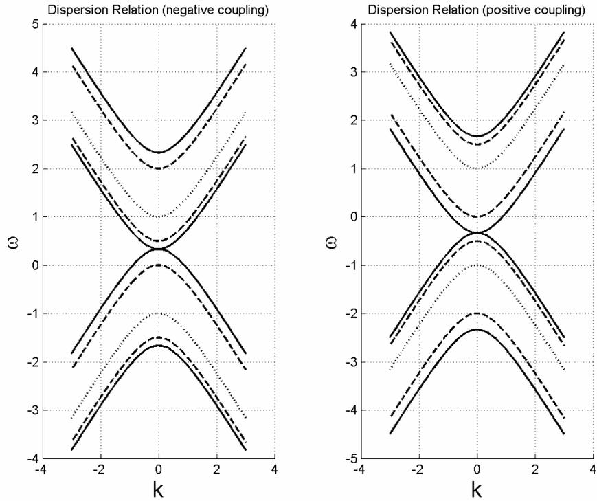
Fig. 1 Dispersion curves for the tri-core system. (a) Zero or negative values of the inter-core coupling constant,  $\lambda = 0$  (dotted),  $\lambda = -0.5$  (dashed), and  $\lambda = -2/3$  (solid). (b) Zero or positive values of the coupling constant:  $\lambda = 0$  (dotted),  $\lambda = 0.5$  (dashed), and  $\lambda = 2/3$  (solid).
