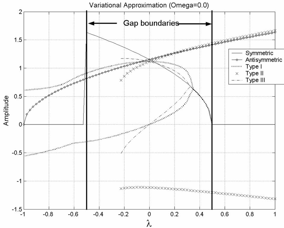
Fig. 3. Amplitudes of different types of solitons, found by means of the variational method, vs. the inter-core solitons  $\lambda$  in the case of  $\omega = 0$ . Note that each symbol forms two different curves, corresponding to amplitudes of two different components of the soliton.
