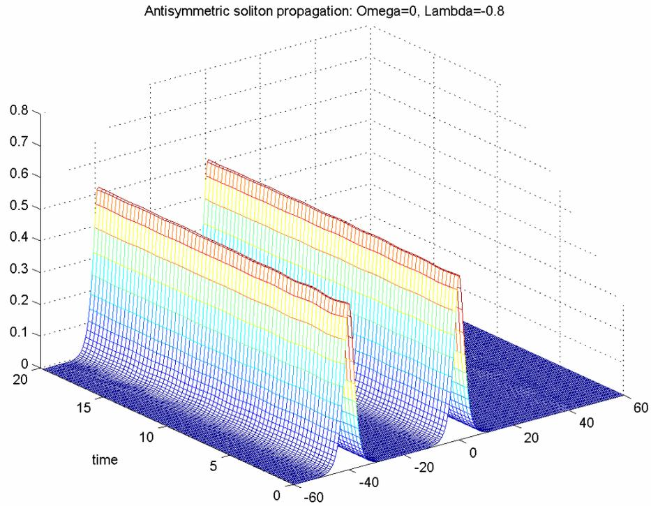
Fig. 8. A typical example of the stable antisymmetric soliton (with one empty core), found *outside* the spectral gap. Three components of the soliton are shown in one panel for the sake of compactness. Small intrinsic oscillations of the soliton observed in the figure are due to initial perturbations added to the soliton.
