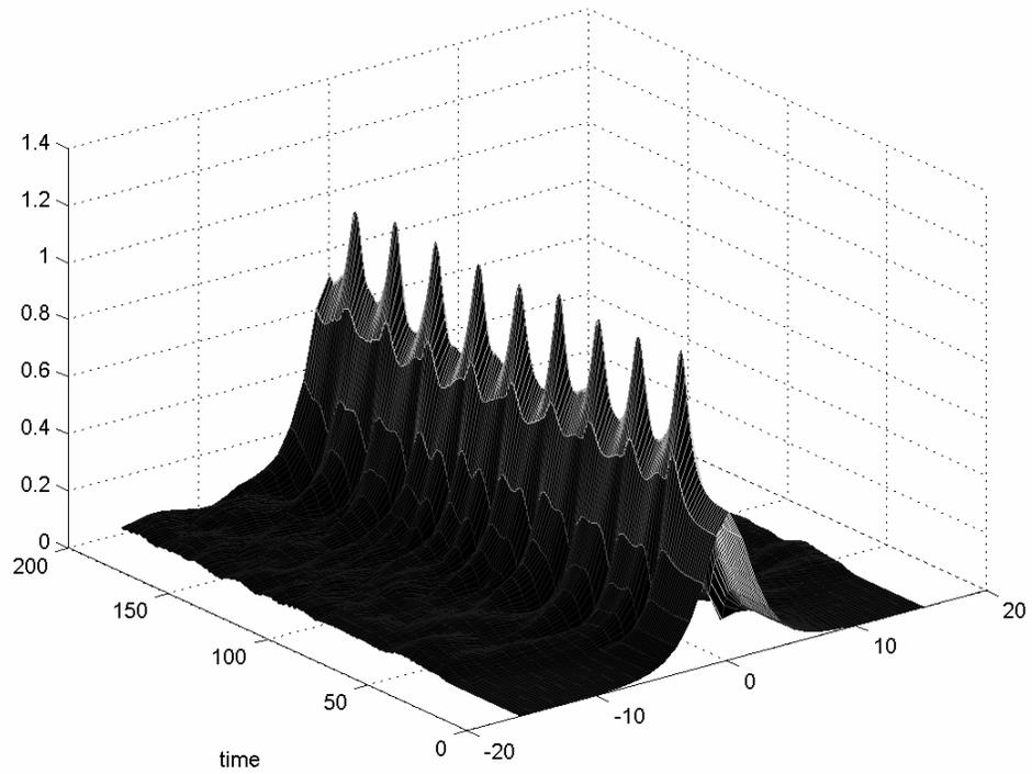
Fig. 12. Transformation of an unstable symmetric soliton into a breather by the oscillatory instability in the dual-core system, in the case of  $\omega = 0.6$ ,  $\lambda = 0.2$ . After a transient period, the vibrations settle down to a quasi-steady state.
