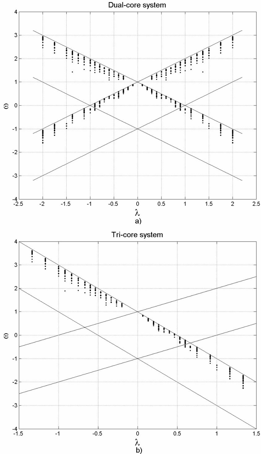
Fig. 10. The stability region of symmetric solitons: dots mark parameter sets  $(\omega, \lambda)$  for which it was checked that all the eigenvalues of small perturbations around the soliton are stable: (a) the dual-core system (this panel also includes the stability region for the antisymmetric solitons); (b) the tri-core system. The parallel lines with the negative and positive slope are existence borders for the symmetric and antisymmetric solitons, respectively.
