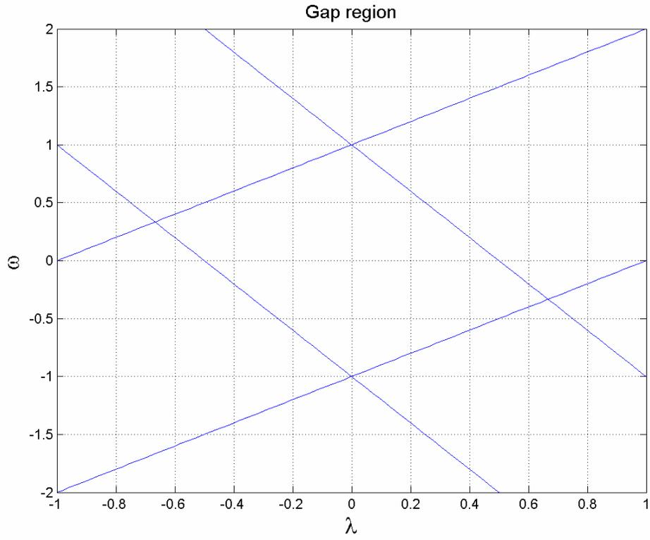
Fig. 2. The region in the parametric plane  $(\lambda, \omega)$  of the system of three linearly coupled Bragg gratings where the spectral gap exists. Two stripes are defined by Eqs. (3.3) and (3.4). The genuine gap is the rhombus formed by intersection of the stripes.
