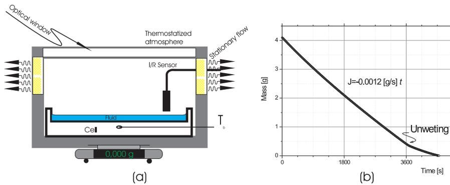
Fig. 1 (a) Scheme of the experiment: a cylindrical cell is mounted in a closed environment where a very small flow refresh air and vapor pressure. (b) The pressure unbalance drive an almost linear evaporation rate until the drying process begins.
